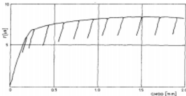
**Figure 1:** Load  $F$  vs. crack mouth opening displacement CMOD relationship, obtained for stable crack growth by single specimen unloading compliance technique for J integral testing
