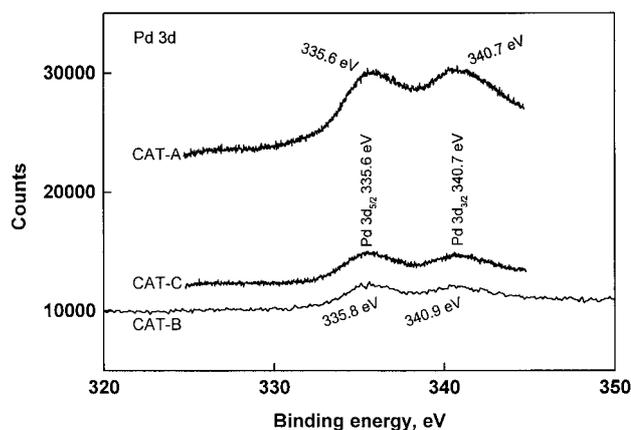
**Figure 2:** XPS Pd 3d spectra of reduced catalysts
