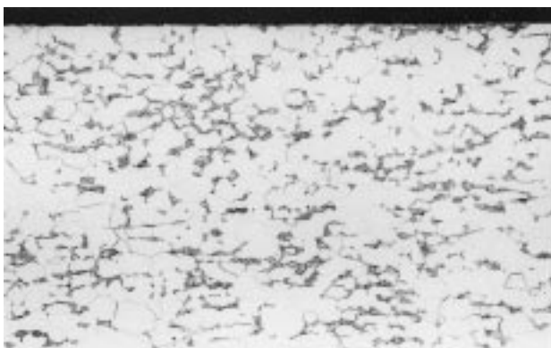
Figure 2: Ferrite-pearlite microstructure of alloy No.6 (with 0.048 wt.% Sb) after decarburization ( p(\text{H}_2\text{O})/p(\text{H}_2)=0.03 , t=15 min, T=840^\circ\text{C} , M 500x, Nital)
