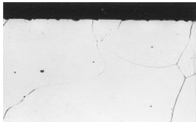
Figure 4: Ferrite microstructure of alloy No.4 after decarburization ( p(\text{H}_2\text{O})/p(\text{H}_2)=0.03 , t=15 min, T=840^\circ\text{C} , M 500x, Nital)
