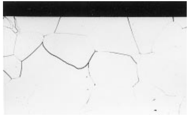
Figure 3: Ferrite microstructure of alloy No.3 (with 0.048 wt.% Sb) after decarburization ( p(\text{H}_2\text{O})/p(\text{H}_2)=0.03 , t=15 min, T=840^\circ\text{C} , M 500x, Nital)
