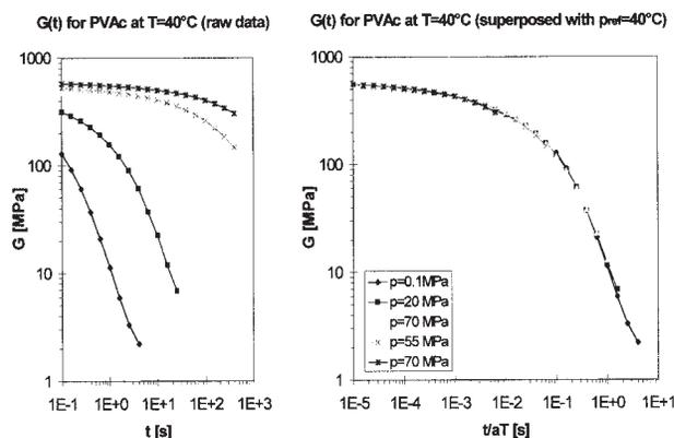
**Figure 4:** Shear modulus for PVAc at various pressures
