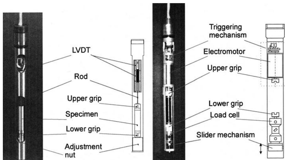
Figure 2: Insert for volume and shear relaxation measurements
