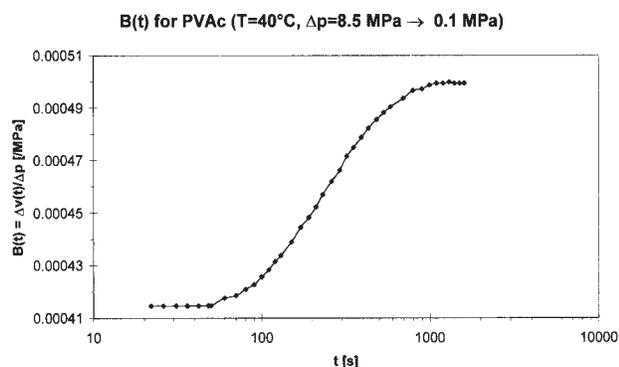
**Figure 3:** Bulk Creep Compliance  $B(T)$  for PVAc at 40C subjected to a pressure drop from 8.5 MPa to 0.1 MPa
