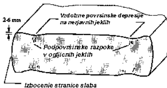
Slika 1: Lokacija depresij in razpok na kontilitem slabu Figure 1: Surface depressions and cracks on continuous casting slab
