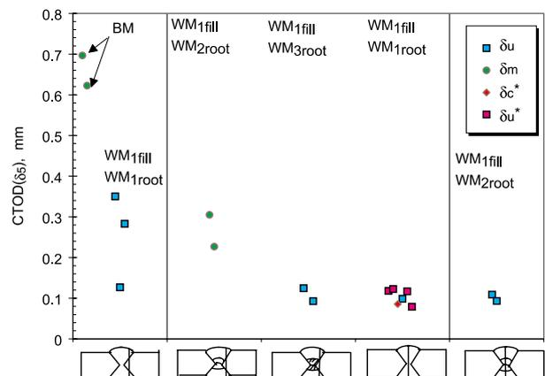
**Figure 5:** CTOD( $\delta_5$ ) values for specimens with the crack front through the HAZ and WM in the over-matched weld joints, measured at  $-10\text{ }^\circ\text{C}$
