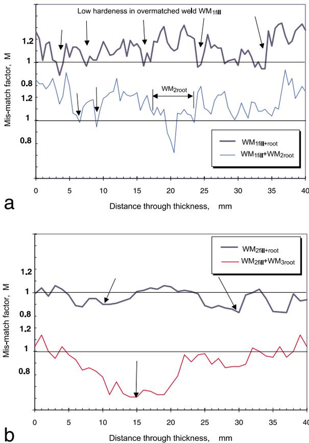
**Figure 3:** Mis-match distribution across the midthickness of a) over-matched, b) under-matched weld joint
