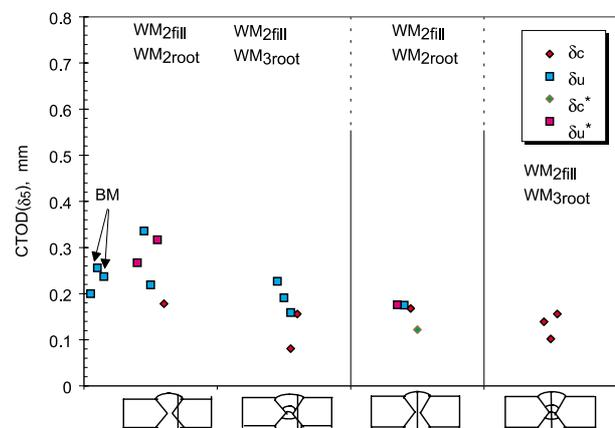
**Figure 8:** CTOD( $\delta_5$ ) values for specimens with the crack front through the HAZ and WM in the under-matched weld joints, measured at  $-10\text{ }^\circ\text{C}$
