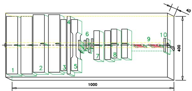
**Figure 2:** Specimens sampled in welded plates
