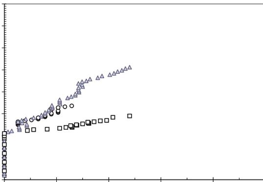
**Figure 9:** Comparison of R curves for HAZ and WM of homogeneous and heterogeneous undermatched weld joints
