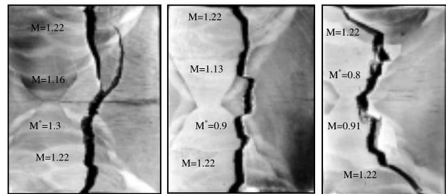
**Figure 7:** The crack growth path deviation of cleavage crack propagation on the macro-etch sectioning 8 mm below of fatigue pre-crack front, as the consequence of global/local mis-matching
