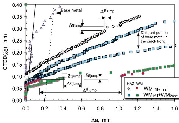
**Figure 6:** CTOD-R resistance curves for specimen with the crack front through the HAZ (crack depth  $a/W=0.5$ ) and WM in the over-matched weld joints
