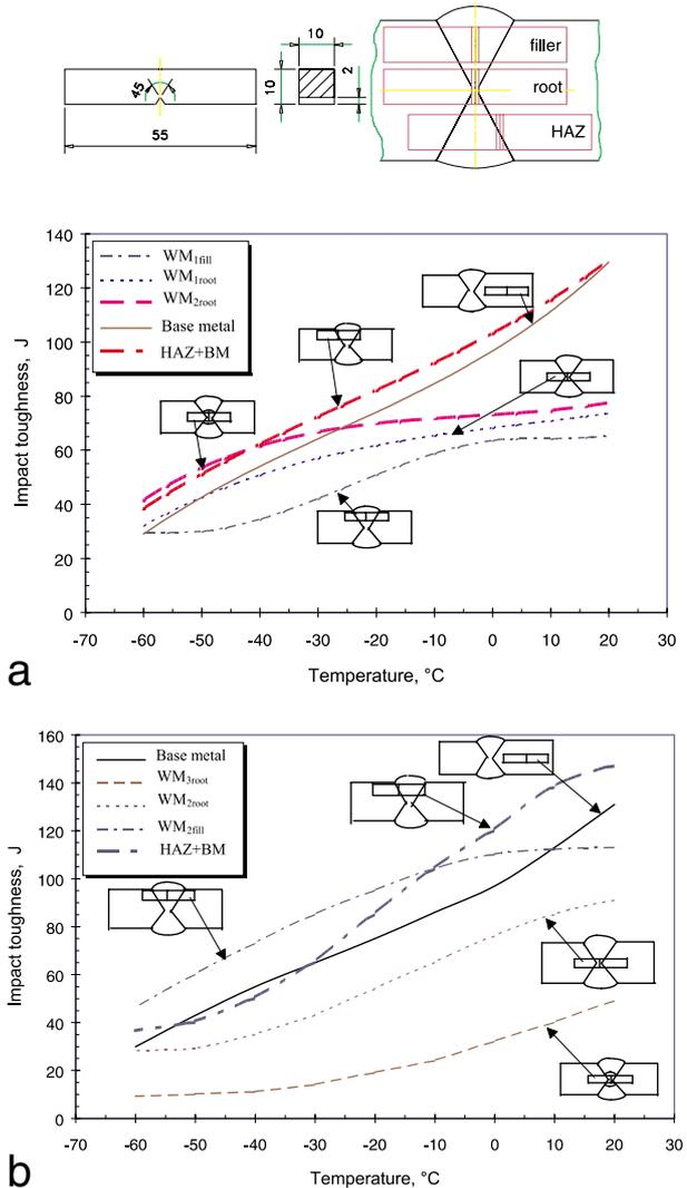
**Figure 4:** Impact toughness transition curves for a) over-matched b) under-matched weld joint
