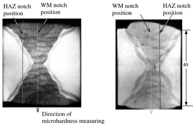
**Figure 1:** Weld joints cross-sections
