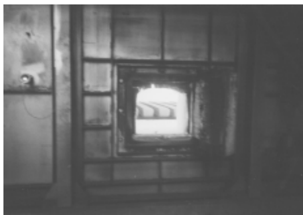
Slika 3: Stranska vrata peči in razmestitev gredic Figure 3: Side-wall door and billets arrangement
