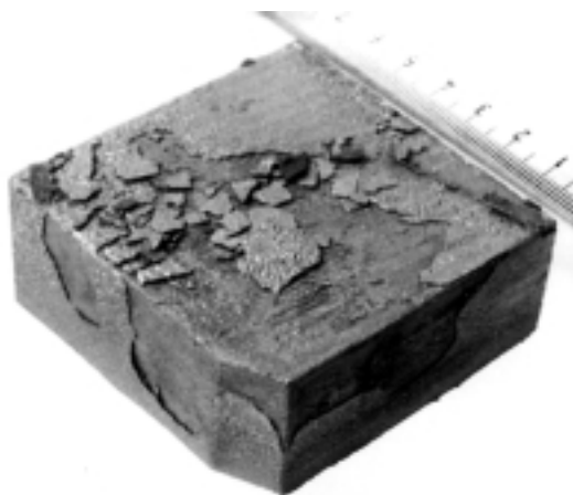
Slika 10: Škaja po optimizaciji (vzorec 2) Figure 10: Scale after optimization (speciment 2)
