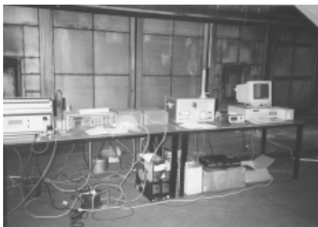
Slika 2: Prenosni merilni sistem za analizo plinov Figure 2: Portable measuring set-up for data acquisition
