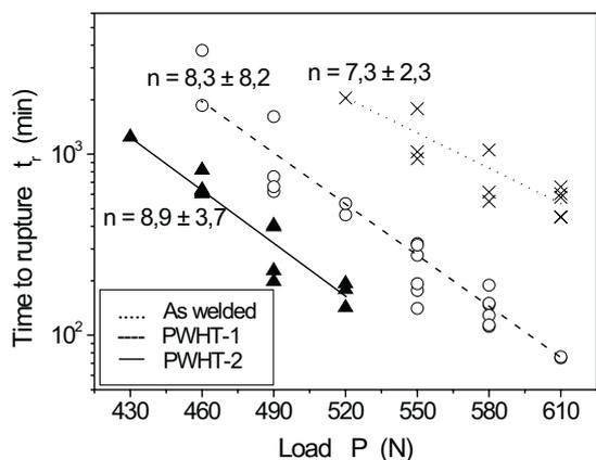
**Figure 5:** Load exponent  $n$  for P91 steel weldments in three different heat-treatment conditions
