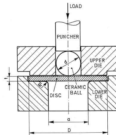
**Figure 2:** Schematic illustration of the dies in the small-punch test equipment
