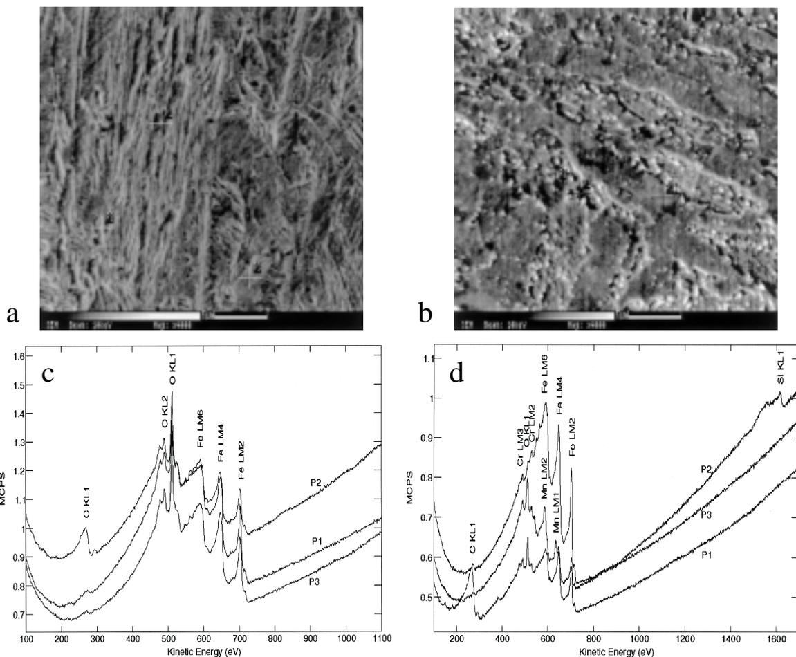
**Figure 7:** HRAES spectra of as-welded and crept specimens of P91 steel weldment shows chromium peaks that indicate a carbide precipitation process: a) SEM, as-welded, b) SEM, as-welded after 2040 min creep test, c) HRAES, as-welded, d) HRAES, as-welded after 2040 min creep test
