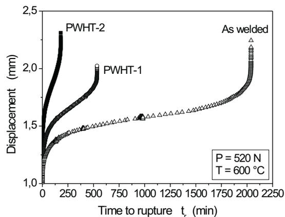
**Figure 6:** Time dependence of the central disc displacement in the small-punch test for the P91 steel weldment for three different heat-treatment conditions
