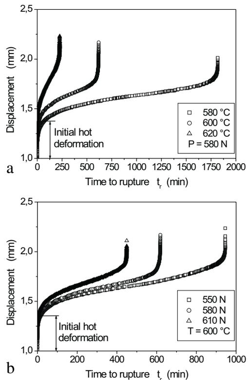
**Figure 4:** Central disc displacement vs. time in the small-punch test at different temperatures and loads. The P91 steel weldment is in the as-welded condition. a)  $P = \text{const.} = 580 \text{ N}$ , b)  $T = \text{const.} = 600 \text{ °C}$
