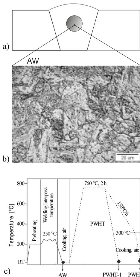
**Figure 1:** P91 steel weldment: a) Schematic presentation of pure weld and location of the specimens, b) The microstructure in the as-welded condition (AW), c) Welding parameters
