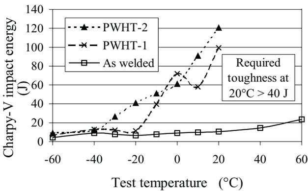
**Figure 3:** Charpy-V impact energy of P91 steel weldments
