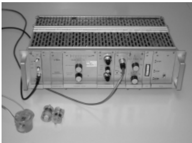
Slika 6: Protonski magnetometer s sondami Figure 6: Proton magnetometer with probes
