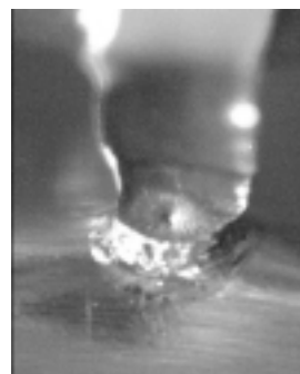
Slika 6: Fotografija dobrega zvara po nateznem preizkusu Figure 6: Photograph of a good weld after the tearing test
