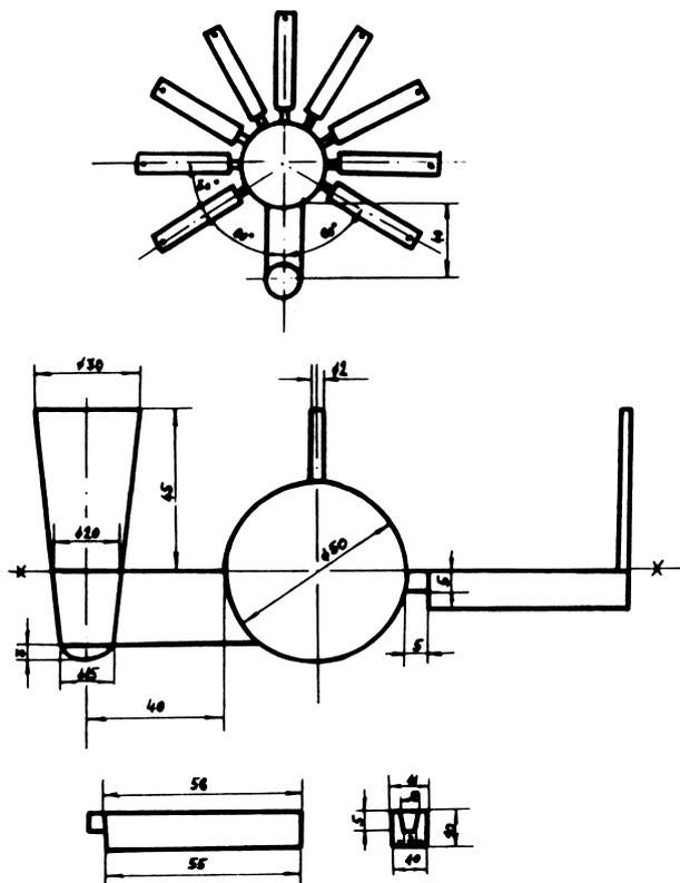
**Figure 1:** Drawing and dimensions of the cast pieces for impact-resistance testing with the gating and risering systems
