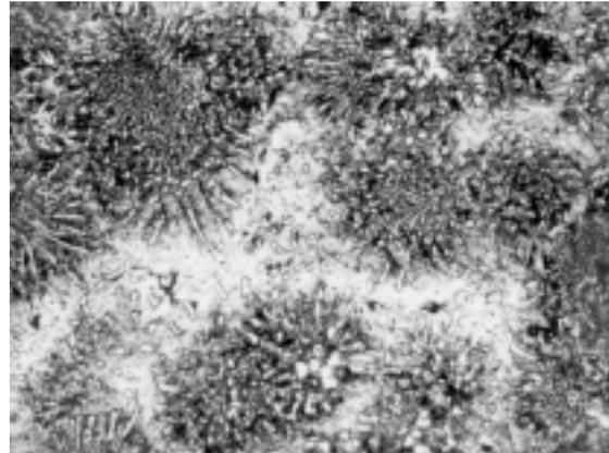
**Figure 12:** Microstructure of a white cast-iron sample, heat no. 5 with 11.32 wt. % vanadium, in heat-treated condition, nital etched, 500x
