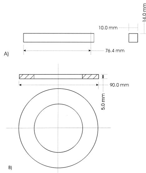
**Figure 2:** Drawing and dimensions of samples for testing of a) microstructure and hardness, and b) wear resistance
