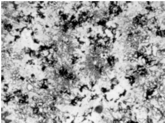
**Figure 11:** Microstructure of a white cast-iron sample, heat no. 4 with 8.72 wt. % vanadium, in heat-treated condition, nital etched, 500x
