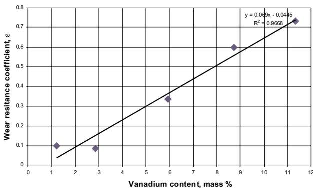
**Figure 14:** The effect of vanadium content in vanadium-alloyed, white cast-iron samples on the abrasion wear-resistance coefficient
