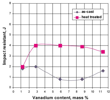
**Figure 13:** The effect of vanadium content on the impact resistance of as-cast and heat-treated white cast-iron samples, tested without notch
