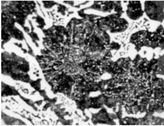
**Figure 10:** Microstructure of a white cast-iron sample, heat no. 2 with 2.86 wt. % vanadium, in heat-treated condition, nital etched, 500x
