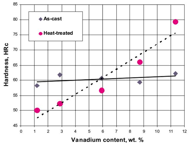
**Figure 4:** The effect of vanadium content on the hardness properties of white cast-iron samples in the as-cast and heat-treated conditions
