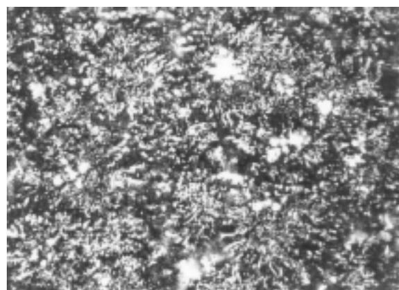
**Figure 8:** Microstructure of a white cast-iron sample, heat no. 5 with 11.32 wt. % vanadium, in as-cast condition, nital etched, 500×
