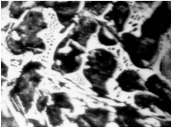
**Figure 5:** Microstructure of a white cast-iron sample, heat no. 1 with 1.2 wt. % vanadium, in as-cast condition, nital etched, 500×
