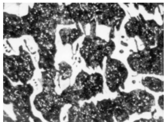
**Figure 9:** Microstructure of a white cast-iron sample, heat no. 1 with 1.2 wt. % vanadium, in heat-treated condition, nital etched, 500×
