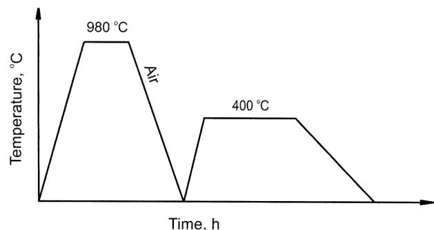
**Figure 3:** Schematic presentation of the heat-treatment procedure of vanadium-alloyed white cast irons
