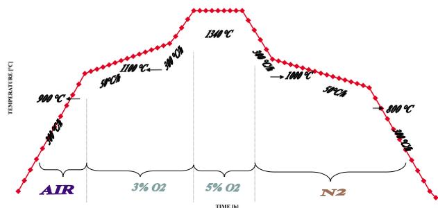
Figure 4: Typical firing scheme for the sintering of high-performance power ferrites
