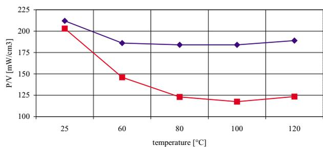
**Figure 2:** Core loss as a function of temperature at 400 kHz and 50 mT (measured for toroids of dimensions:  $d_0 = 22$  mm,  $d_i = 14$  mm,  $h = 7$  mm) for the standard material A and the new design B
