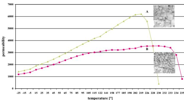
Figure 3: Initial permeability vs. temperature for the standard material A and the new design B
