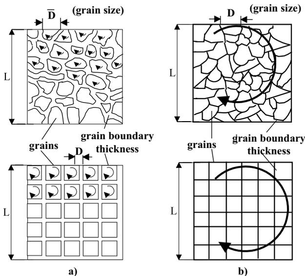
**Figure 1:** Brick-wall-microstructure model: (a) schematic picture of a real and an ideal microstructure of a material with isolated magnetic grains exposed to micro-eddy currents. (b) a sketch of an actual and an idealised ferrite microstructure with grain boundaries permeable to the eddy current.
