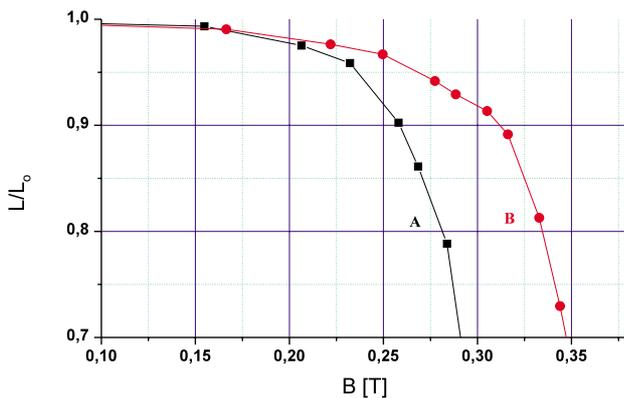
**Figure 5:** Inductance of toroid cores with an air-gap, made from the standard material, A, and the new design, B, as a function of  $B_{PK\_MAX}$  at 120 °C
