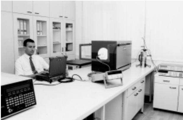
Laboratorijska peč in merilni sistem za visokotemperaturno umerjanje termoelementov (do 1300 °C) in simulacijski model ogrevanja za vsako gredico v realnem času (Allino peč – Metal Ravne), razvit na IMT Laboratory furnace and measuring system for the calibration of thermoelements up to 1300 °C and simulation model for the heating of single billets in real time (Allino furnace – Metal Ravne), developed in IMT
