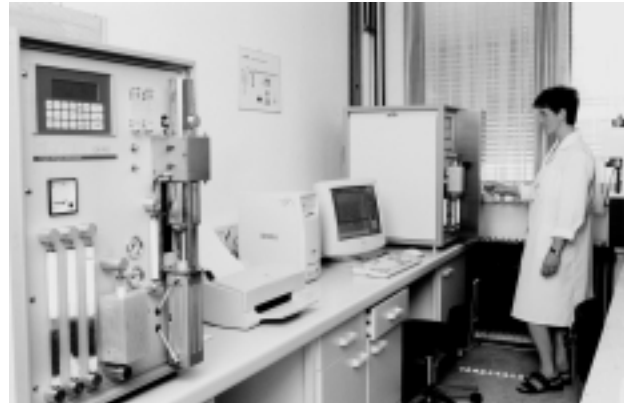
Analizator ogljika in žvepla (ELTRA CS800) ter analizator kisika in dušika (ELTRA ON900) v laboratoriju za analizo kemijo Carbon and sulphur analyser and oxygen and nitrogen analyser in the laboratory of analytical chemistry
