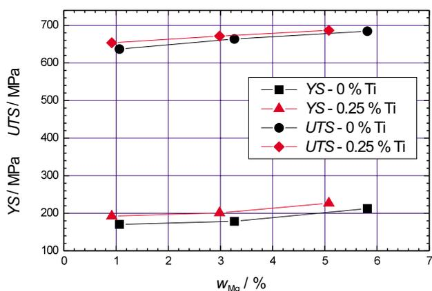
**Figure 14:** Compression strength of AlCuMg alloys with different contents of magnesium and titanium
