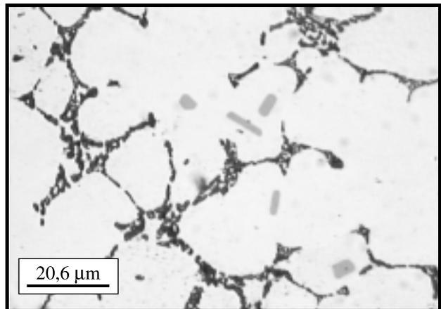
**Figure 6:** Microstructure of the AlCu5Mg5 (0.25 % Ti) alloy (Etched with Keller's reagent)
