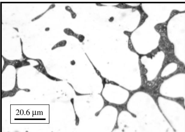
**Figure 3:** Microstructure of the AlCu5Mg3 alloy without Ti addition (Etched with Keller's reagent)
