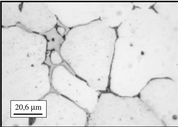
**Figure 2:** Microstructure of the AlCu5Mg1 (0.25 % Ti) alloy (Etched with Keller's reagent)
