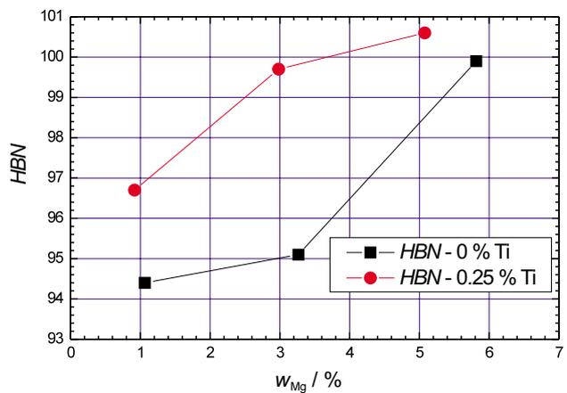
**Figure 13:** Hardness  $HBN$  of the  $\text{AlCuMg}$  alloys with different contents of magnesium and titanium
