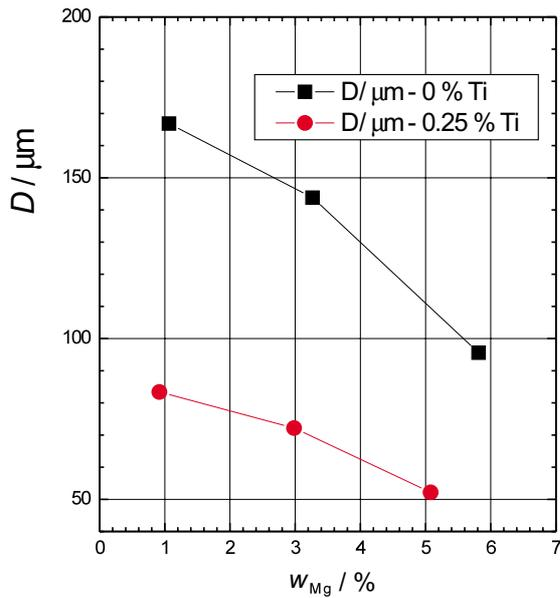
**Figure 7:** Grain size  $D$  for different magnesium and titanium contents in AlCuMg alloys
