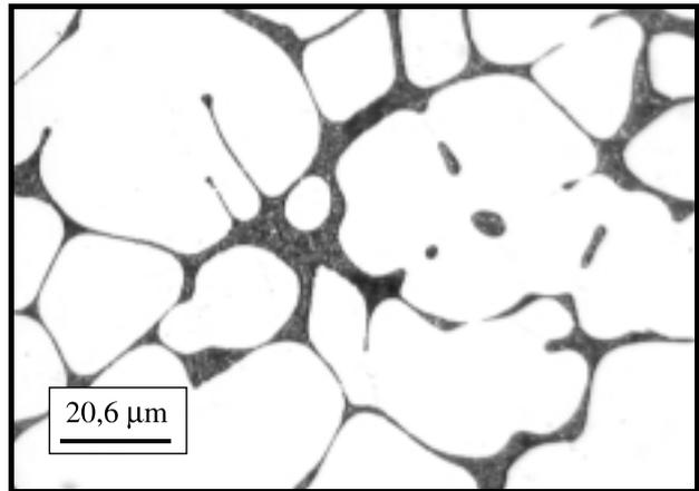
**Figure 4:** Microstructure of the AlCu5Mg3 (0.25 % Ti) alloy (Etched with Keller's reagent)
