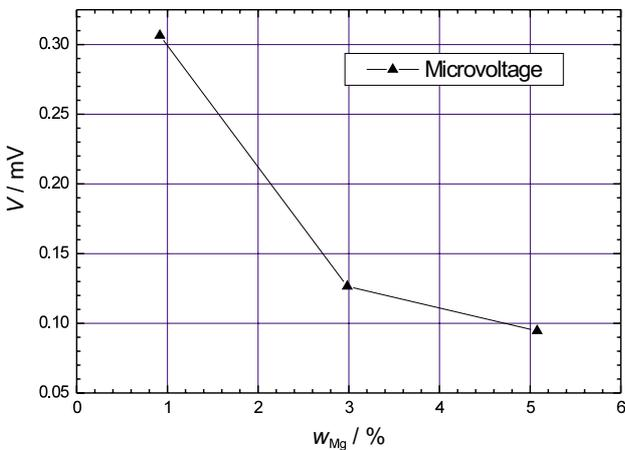
**Figure 11:** The microvoltage  $V$  in the crystallographic direction [112] for different magnesium contents in the alloys with 0.25 % Ti
