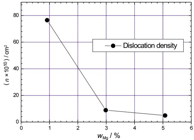
**Figure 12:** Dislocation density  $n$  in the direction [112] for different magnesium contents in the alloys with 0.25 % Ti
