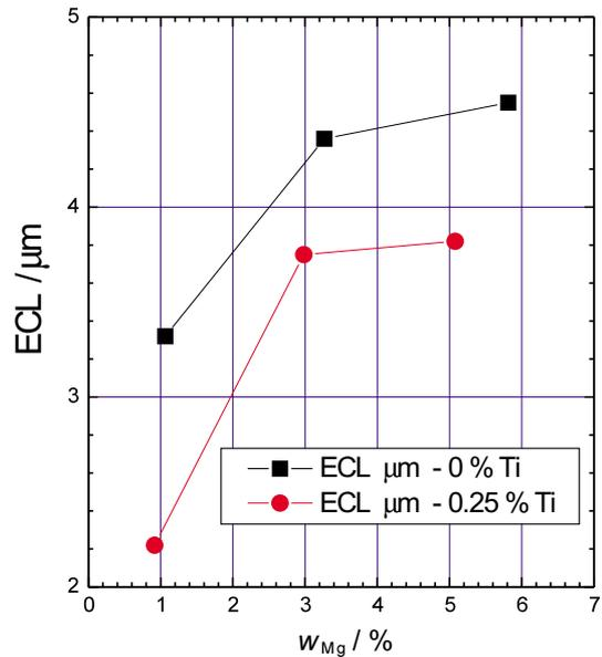
**Figure 9:** Eutectic cell length and volume fraction of eutectic for different magnesium and titanium contents in AlCuMg alloys
