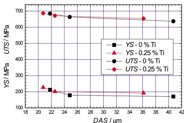
**Figure 15:** Compression strength of AlCuMg alloys in dependence of the secondary dendrite arm spacing (DAS)
