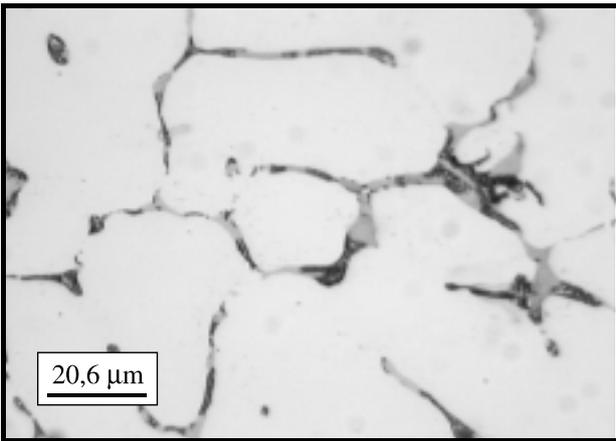
**Figure 1:** Microstructure of the AlCu5Mg1 alloy without any addition of Ti (Etched with Keller's reagent)
