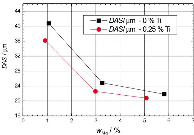
**Figure 8:** Dendrite arm spacing (DAS) for different magnesium and titanium contents in AlCuMg alloys
