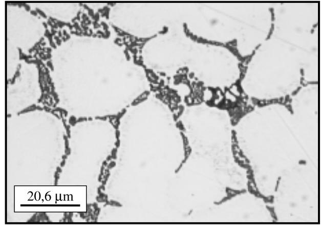
**Figure 5:** Microstructure of the AlCu5Mg5 alloy without Ti addition (Etched with Keller's reagent)
