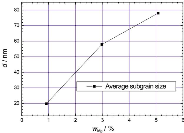
**Figure 10:** Average sub-grain size ( $d/\text{nm}$ ) in the crystallographic direction [112] for different magnesium contents in the alloys (0.25 % Ti)
