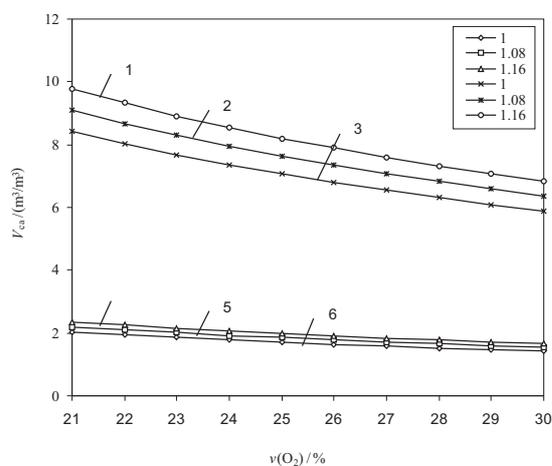
**Figure 1:** Effect of oxygen content in the combustion air on the amount of air ( $\lambda = 1.10; 1.08; 1.16$ ); 1, 2, 3 - Natural gas; 4, 5, 6 - Mixed gas
