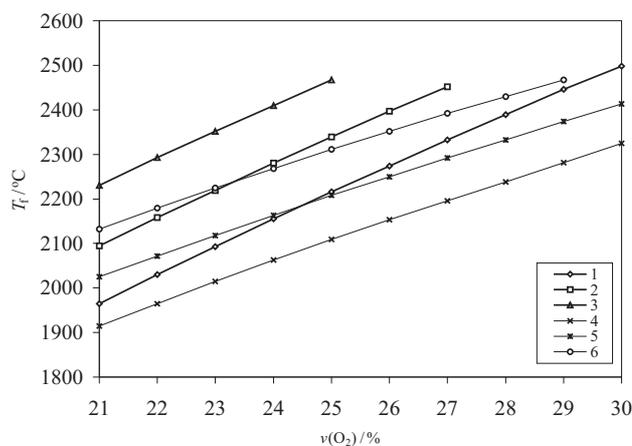
**Figure 5:** Influence of air oxygen content on flame temperature ( $\lambda = 1.10$ ); 1, 2, 3 – Natural gas; 4, 5, 6 – Mixed gas; 1, 4 ( $T_{ca} = 100\text{ °C}$ ); 2, 5 ( $T_{ca} = 300\text{ °C}$ ); 3, 6 ( $T_{ca} = 500\text{ °C}$ )
