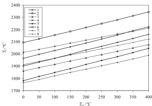
**Figure 3:** Changes in flame-temperature values with air preheat temperature 1, 2, 5, 6 – Natural gas; 3, 4, 7, 8 – Mixed gas; 1, 3 ( $\lambda = 1.10$ ,  $v(O_2) = 21\%$ ); 2, 4 ( $\lambda = 1.10$ ,  $v(O_2) = 24\%$ ); 5, 7 ( $\lambda = 1.20$ ,  $v(O_2) = 21\%$ ); 6, 8 ( $\lambda = 1.20$ ,  $v(O_2) = 24\%$ )
