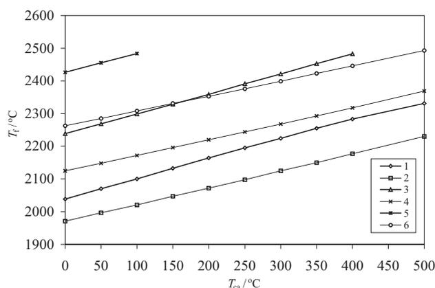
**Figure 4:** Influence of air preheating on flame temperature ( $\lambda = 1.10$ ); 1, 3, 5 – Natural gas; 2, 4, 6 – Mixed gas; 1, 2 ( $v(O_2) = 21\%$ ); 4, 6 ( $v(O_2) = 24\%$ ); 3, 5 ( $v(O_2) = 27\%$ )
