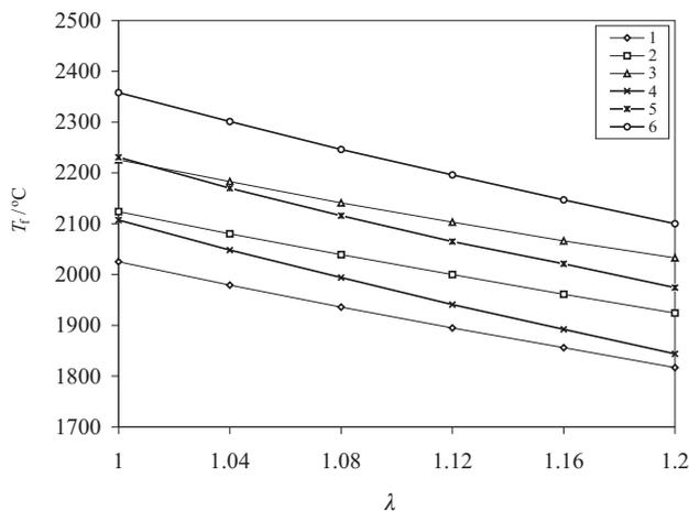
**Figure 6:** Influence of excess air ratio on flame temperature ( $v(\text{O}_2) = 21\%$ ); 1, 2, 3 – Mixed gas; 4, 5, 6 – Natural gas; 1, 4 ( $T_{ca} = 0\text{ }^\circ\text{C}$ ); 2, 5 ( $T_{ca} = 200\text{ }^\circ\text{C}$ ); 3, 6 ( $T_{ca} = 400\text{ }^\circ\text{C}$ )
