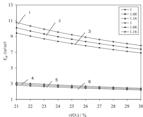
**Figure 2:** Effect of oxygen content in the combustion air on the amount of combustion products ( $\lambda = 1.10; 1.08; 1.16$ ); 1, 2, 3 - Natural gas; 4, 5, 6 - Mixed gas
