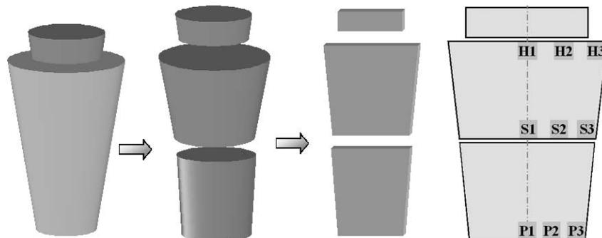
**Figure 5:** Steel ingot dividing and sampling diagram
