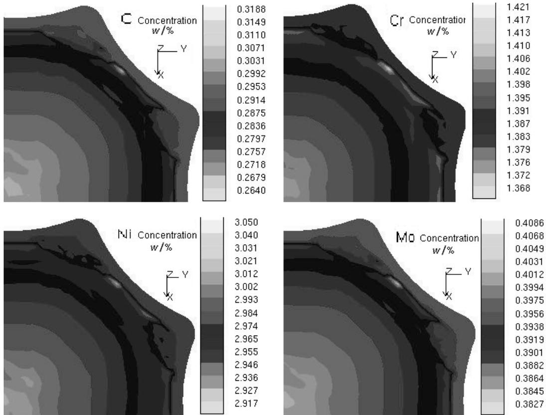
Cross-section view below the ingot top
