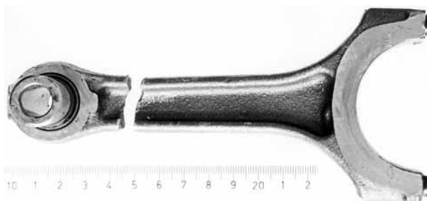
Figure 1: Connecting rod's fractured shank Slika 1: Prelomljeno steblo ojnice
