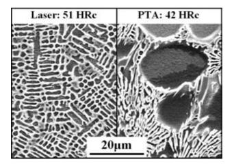
Figure 2: Microstructure of the Stellite 6 layers
