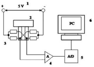
**Figure 1**: Measuring system; 1 – source of electricity, 2 – punch, 3 – strain gauges connected in full Weatstonov bridge, 4 – amplifier, 5 – converter of impulse, 6 – personal computer.
