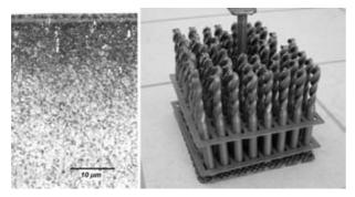
Figure 3: Microstructure and view of screw-taps in furnace equipment after nitrooxidation AG made of SW7M steel
