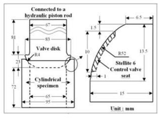
Figure 1: Schematic diagram of the impact wear test
