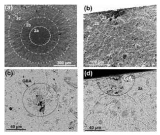
**Figure 1:** Zones of fatigue crack nucleation and propagation in (a), (c) internal and (b), (d) near-surface failures
