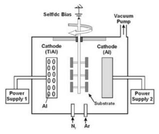
Figure 1: Schematic representation of magnetron sputtering system
