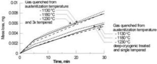
Figure 2. Mass loss by erosion wear of PM S390 MC high speed steel test samples after standard heat treatment and deep-cryogenic treatment
