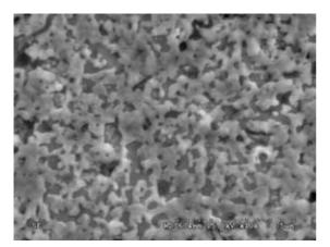
Figure 1: Surface morphology of nitrided layer produced at  $470^{\circ}$ C, for 16h
