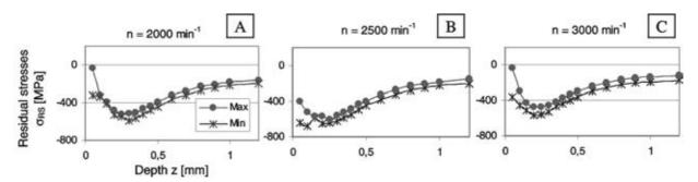
Figure 1: Residual-stress profiles of maraging steel after cold deformation of surface layer and after subsequent precipitation hardening at 450°C for2 hours.
