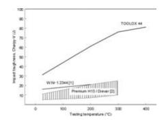
Figure 1: Charpy-V impact toughness in regular grades and in TOOLOX  $44\,$
