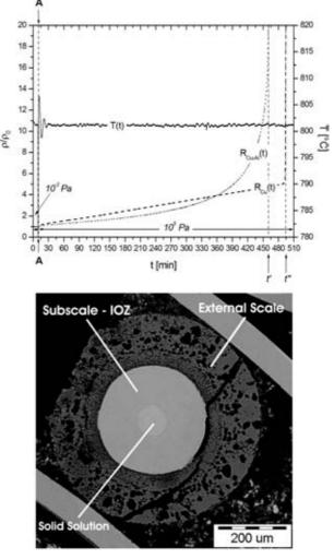
**Figure 1:** Change of electrical resistance during annealing of Cu and Cu-Al alloy at 800°C and Microstructure of partially high – temperature oxidized cylindrical sample of Cu-Al (1.25 at.% Al) alloy at T=800°C and t=240 min.
