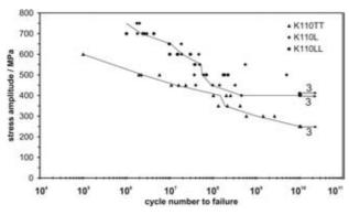
Figure 1: S-N data of AISI D2 type wrought cold work tool steel.
