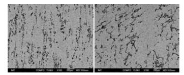
Figure 1: Distribution of carbides (SEM micrographs) in two samples; left: No. 2 (low volume loss) and right: No. 10 (higher volume loss)
