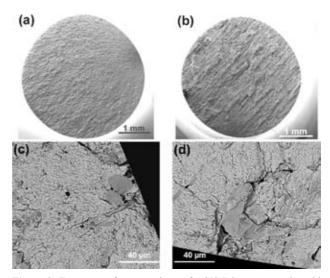
**Figure 2:** Fracture surface overviews of ASIS D2 type wrought cold work tool steel: (a) K110LL, (b) K110TT; primary carbide clusters to be crack origins of (c) K110LL and (d) K110TT specimens.
