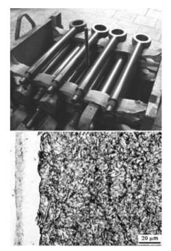
**Figure 1:** View of hydraulics rods oxidation and impregnation after nitriding and microstructure of nitrided 40HM steel (AISI4140)
