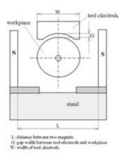
Figure 2: Schematics and configuration of the magnetic-assistance system, tool electrode and workpiece
