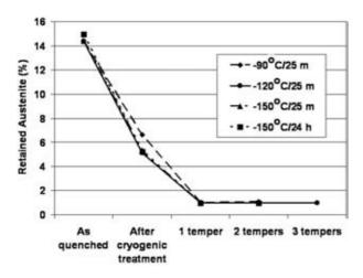
Figure 1: The effect of deep cold treatment on retained austenite
