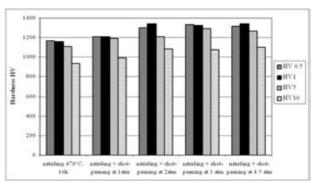
Figure 3: Surface hardness HV0.5, HV1, HV5, HV10 for nitrided layers and surface layers after duplex treatment /nitriding+shot-peening/
