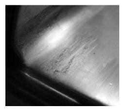
Figure 2: Uncoated t ool corner area after 100 pieces
