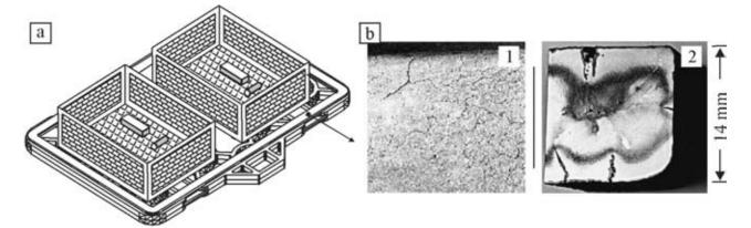
Figure 1: The grate from a carburising chamber furnace withdrawn from use: a) schematic diagram, b) surface cracks (1), macrostructure on the wall cross-section (2) with well visible carburised layer, cracks and axial porosity
