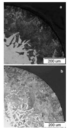
Figure 3: The progress and the morphology of carburized zone after active (a) and passive stage (b) of the process
