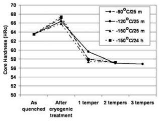
Figure 2: The effect of deep cold treatment on hardness
