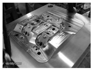
Figure 3: Aluminium pressure die-casting mould
