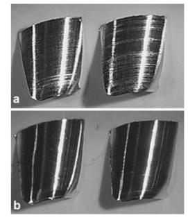
Figure 3: Cutting chips from dry Al machining (a – uncoated tool, b – Cr+WC:h+DLC coated tool)
