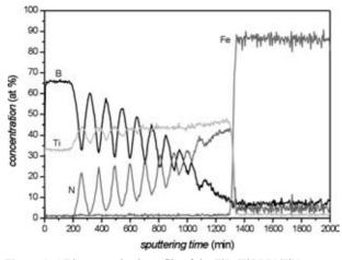
Figure 1: AES sputter depth profile of the TiB<sub>2</sub>/Ti(N-B)/TiN
