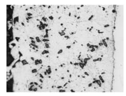
Figure 1: Microstructure of Al12Si/50SiC<sub>8</sub> composite coating
