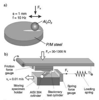
Figure 1: Test setup; (a) pin-disc and (b) load-scanner
