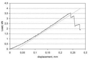
Figure 2: Fracture behaviour of single edge bend specimen
