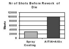
Figure 2: Aluminum die casting results /Diesel Injection pump housing
