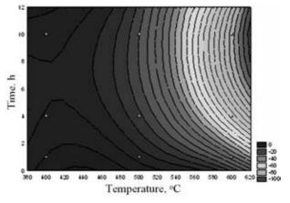
Figure 2: Distribution of dimensional changes of Maraging 15 10 5 steel depending on factors levels
