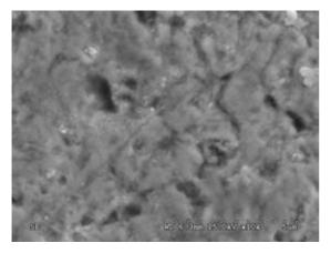
Figure 2: Surface morphology of nitrided layer after shot-peening treatment
