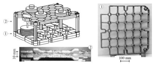
Figure 2: An assembly of grates withdrawn from use in pusher-type furnace: 1) scrap base grate, 2) supporting rod with cracks and deformations
