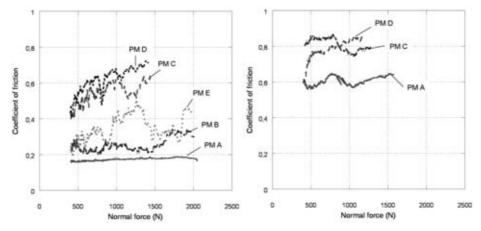
Figure 1: Typical coefficient of friction vs. normal load curves. a) SS against PM A-E b) Al against PM A, C and D.
