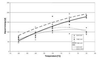
Figure 3: Impact toughness of multipass welds
