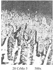
Figure 2: Boride layer photomicrograph
