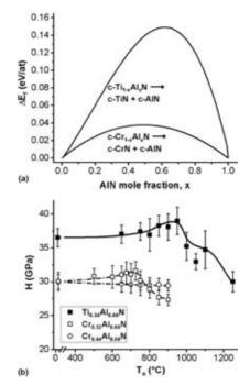
**Figure 2:** (a) Energy of formation difference ( $\Delta E_t$ ) for the separation of c-Ti<sub>1-x</sub>Al<sub>x</sub>N into c-TiN and c-AlN and the separation of c-Cr<sub>1-x</sub>Al<sub>x</sub>N into c-CrN and c-AlN as a function of AlN mole fraction. (b) Hardness (H) of Ti<sub>0.34</sub>Al<sub>0.66</sub>N, Cr<sub>0.32</sub>Al<sub>0.68</sub>N and Cr<sub>0.44</sub>Al<sub>0.56</sub>N as a function of annealing temperature T<sub>a</sub>.
