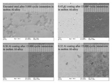
Figure 1: SEM observation of uncoated and coated surface subjected to cyclic immersion in molten alumiunium alloy.
