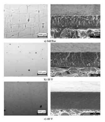
Figure 2: SEM images of coating by using diffirent bias voltage: surface (left) cross section (right)
