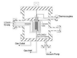
Figure2: Facility for quenching the specimens (proprietary IWT) [2]
