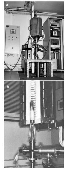
Figure 1: Laboratory device (a) and measurement cell (b) for "in-situ" electrical resistance measurements
