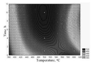
Figure 1: Distribution of hardness values HV1 of Maraging 15 10 5 steel depending on factors levels
