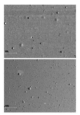
Figure 1: The structure of polishing and nitriding X37CrMoV5-1 steel after ion etching: a) Cr ions (marker  $-10 \ \mu$ m), b) Ti ions (marker  $-10 \ \mu$ m)
