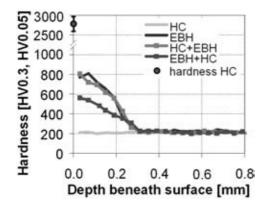
Figure 1: Hardness depth profiles of the combination of HC and EBH
