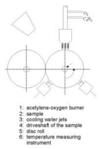
Figure 1: Principle of the apparatus for thermal and mechanical fatigue testing
