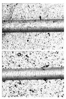
Figure 2: Scratch test on the PVD coat obtain on the nitrided steel: a) CrN coat, b) TiN coat
