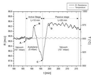
Figure 2: In-situ measurement of electrical resistance changes during vacuum carburizing of the pure iron at  $T=950^{\circ}C$
