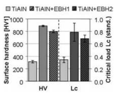
Figure 3: Improvement of surface hardness HV 1 and critical load (standardized values) of TiAlN coatings on C45 (H+T) basic material by subsequent EB hardening
