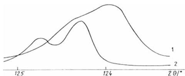
Figure 6: Welded tube. Profile of the diffraction lines (220) for the weld (1) and the base steel (2).
