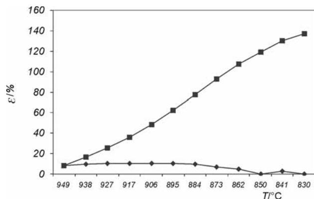
Figure 3: The per-pass (◆) and total (■) reduction of the diameter
