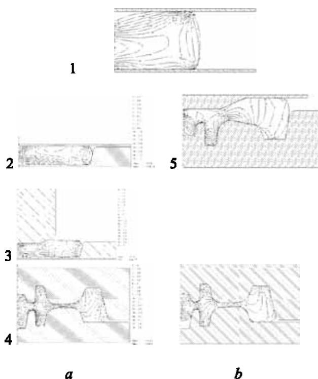
**Figure 1:** Results of the calculation of the wheel-blank shape change at different stages of the existing (a) and the experimental (b) technology: 1 – upsetting in the 20-MN press; 2 – upsetting to a ring in the 50-MN press; 3 – ring expansion (dilatation) with a punch on the 50-MN press; 4 – stamping in the 100-MN press; 5 – stamping in the 50-MN press
