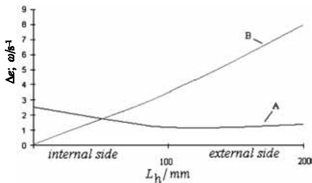
**Figure 3:** Distribution of the degree (A) and the rate (B) of steel deformation along the generatrix of the wheel-hub bore for stamping the blank in the 100-MN press
