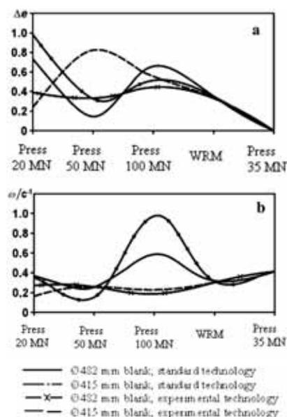
**Figure 2:** Distribution of deformation (a) and of deformation rate (b) in the central wheel-rim zone for the stages of the blanks' forming using different schemes of stamping
