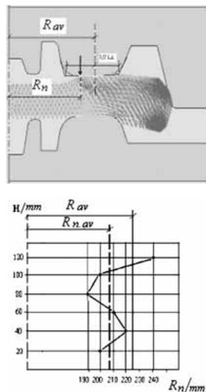
**Figure 4.1:** Variation of the position of the neutral plane ( $R_n$ ) relative to the middle of the disc ( $R_{av}$ ) in the process of forming the wheel blank with  $D = 957 \text{ mm}$  in the 100-MN press
