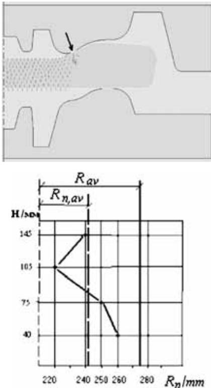
**Figure 4.2:** Change of the neutral plane position ( $R_n$ ) relative to the middle of the disc ( $R_{av}$ ) in the process of forming the wheel blank with  $D = 932$  mm in the 100-MN press
