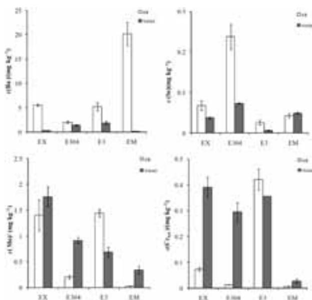
**Figure 2:** Results of the leaching test of minor elements (Ba, Se, Mo, Cr) in air and water cooled EAF slags in  $\text{mg kg}^{-1}$ . Results are presented as the mean value of triplicate analysis with the standard deviation as error bars.
