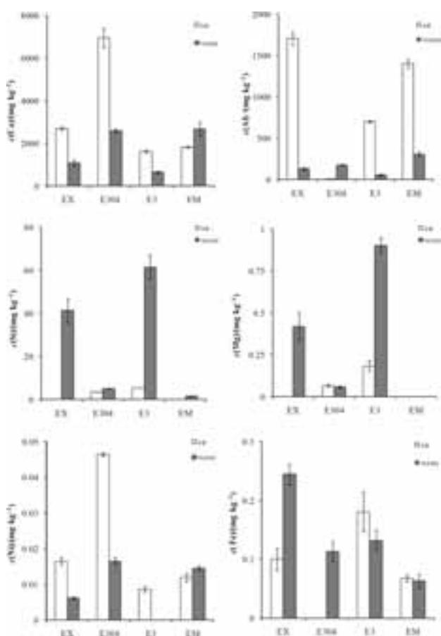
**Figure 1:** Results of the leaching test of major elements in air and water cooled EAF slags in  $\text{mg kg}^{-1}$  (Ca, Al, Si, Mg, Ni, Fe). Results are presented as the mean value of triplicate analysis with the standard deviation as error bars. Values that are not presented in the Figure are under the limit of detection; for Mg ( $0.05 \text{ mg kg}^{-1}$ ); for Si ( $0.1 \text{ mg kg}^{-1}$ ); for Ni ( $0.005 \text{ mg kg}^{-1}$ ); for Fe ( $0.025 \text{ mg kg}^{-1}$ ).
