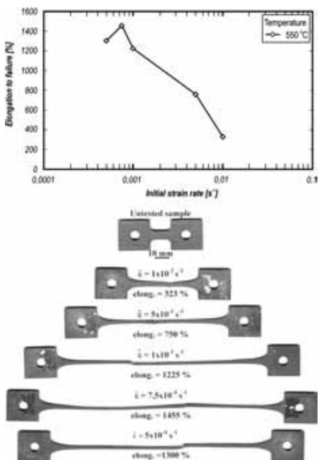
**Figure 4:** Elongation to failure as a function of initial strain rate and the samples after tensile testing at 550 °C
