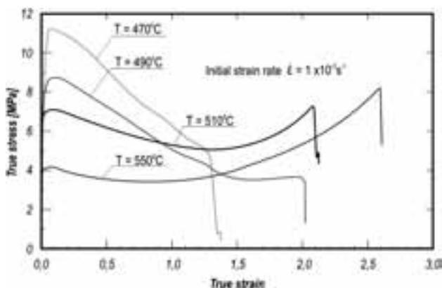
**Figure 1:** True-stress, true-strain curves for various tested temperatures at an initial strain rate of  $1 \times 10^{-3} \text{ s}^{-1}$  (CCHS test)
