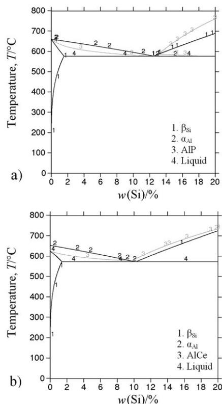
**Figure 2:** Isoleth diagram of AlSi17 alloy with 80 µg/g (ppm) P (a), and the mass fraction of Ce  $w(\text{Ce}) = 4.5\%$  (b)
