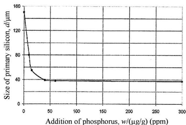
**Figure 1:** Influence of phosphorus additions on the refinement of primary silicon particles<sup>7</sup>
