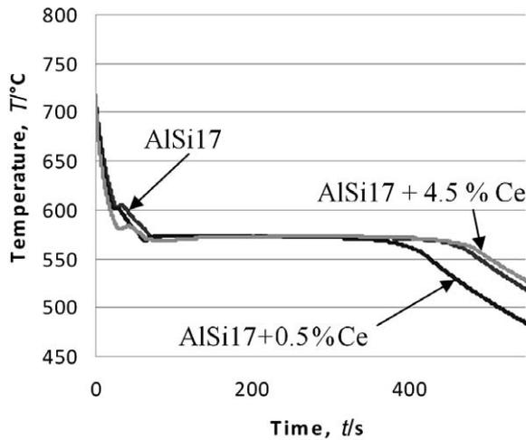
**Figure 3:** Effect of cerium addition on the AISi17 alloy
