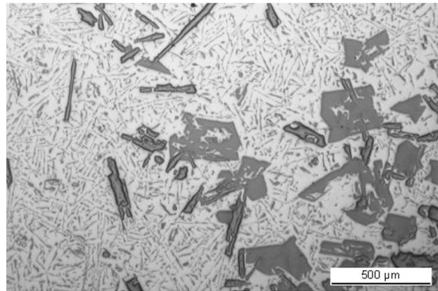
**Figure 5:** AISi17 alloy with  $w = 4.5\%$  Ce
