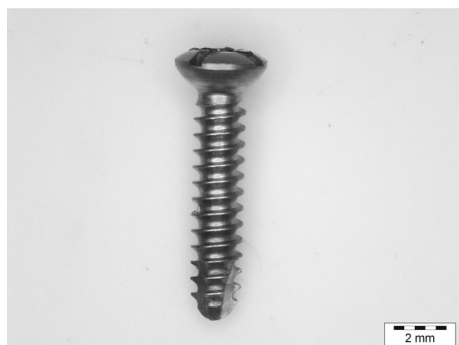
Figure 1: Titanium screw – rejected implant
