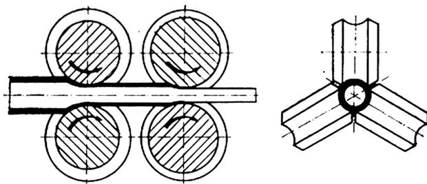
Figure 2: Scheme of the work of the stretch reducing mill<sup>2</sup>
