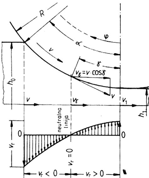
**Figure 5:** Processing rates in the deformation zone (10)
