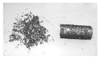
Figure 2: Separated stainles steel chips and compacted, cold pressed chips
