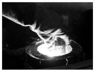
Figure 4: Charging of compact into melt Slika 4: Dodajanje stisnjencev v talino
