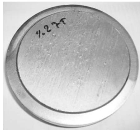
**Figure 6:** Defective ring carrier
