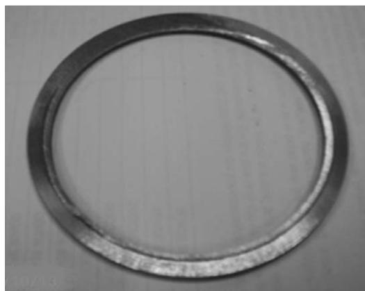
**Figure 1:** Non-defective ring carrier
