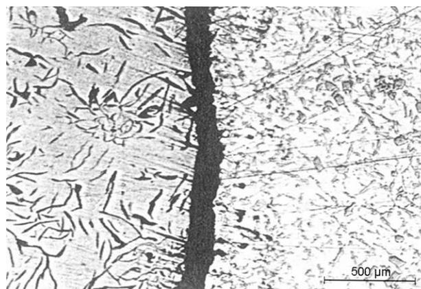
**Figure 2:** Microstructure of ring carrier (100X)
