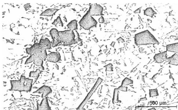
**Figure 3:** Microstructure of ring carrier (Insufficient Si thinning) (100X)
