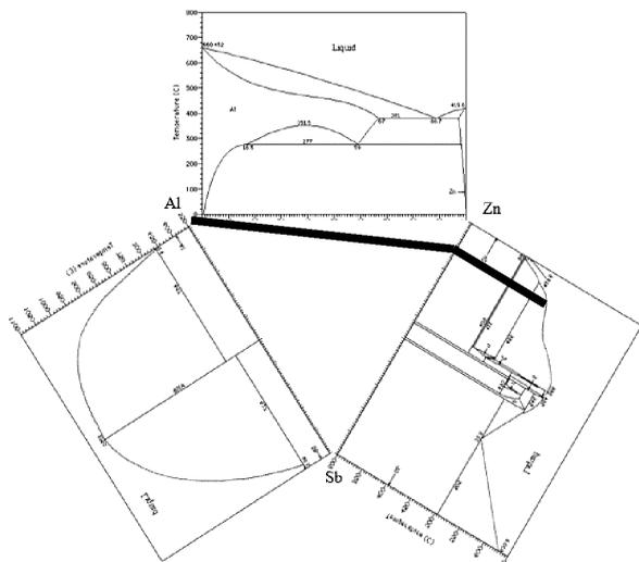
**Figure 1:** Experimental investigation of the section line with the ratio  $w(\text{Zn}) : w(\text{Sb}) = 9 : 1$
