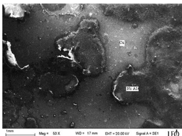
**Figure 1:** SEM images of a metallographic section of the Cu-10 wt % Ni<sub>3</sub>Al composite.
