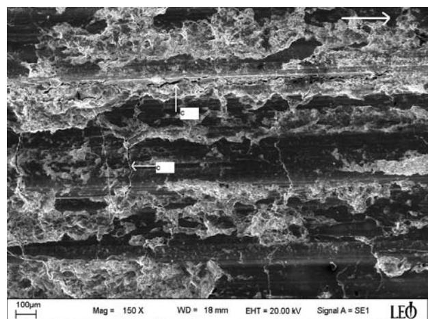
**Figure 6:** SEM images of the worn surfaces of Cu-15 wt. % Ni<sub>3</sub>Al composite at 150 N (“c” showed cracks). The arrow indicates the sliding direction.
