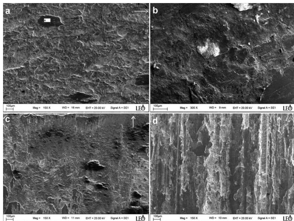
**Figure 4:** SEM images of the worn surfaces: (a) unreinforced Cu matrix tested at 83 N; (b) unreinforced Cu matrix tested at 150 N; (c) Cu-10 wt. % Ni<sub>3</sub>Al composite tested at 83 N; and (d) Cu-10 wt. % Ni<sub>3</sub>Al composite tested at 150 N. The arrow indicates the sliding direction.
