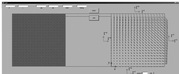
**Figure 3:** Simulation of flat rolled (180 × 180) mm cross sectioned 16MnCrS5 steel at 1100 °C with Young's modulus  $E = 97362.21$  MPa and Poisson's ratio  $\nu = 0.35678$ . The total reduction is 16.66 % and preliminary analyzed with 5 slices by using elastic stiffness matrix <sup>7</sup>. Arrows represents the displacement vector for each slice. The exit speed is equal to 1.14389 times the entry speed of the billet. Due to symmetry only the top right part of the billet is considered.
