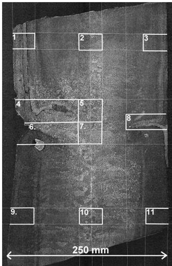
**Figure 1:** Macrostructure of breakout
