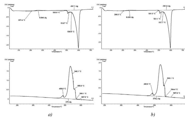
**Figure 4:** Heating and cooling DCS curves of AlSi9Cu3 alloy without Ce (a) and with  $w = 0.02\%$  Ce (b)
