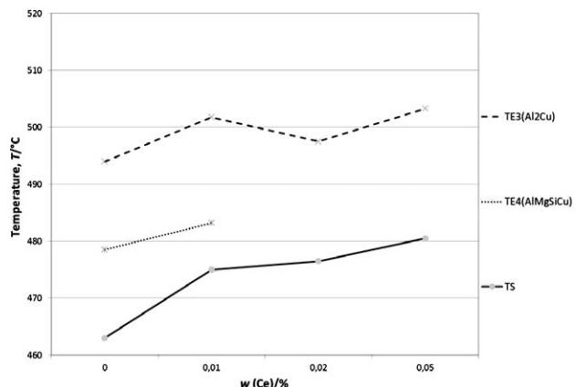
**Figure 3:** Comparison of some characteristic solidification temperatures for AlSi9Cu3 alloy with respect to Ce addition
