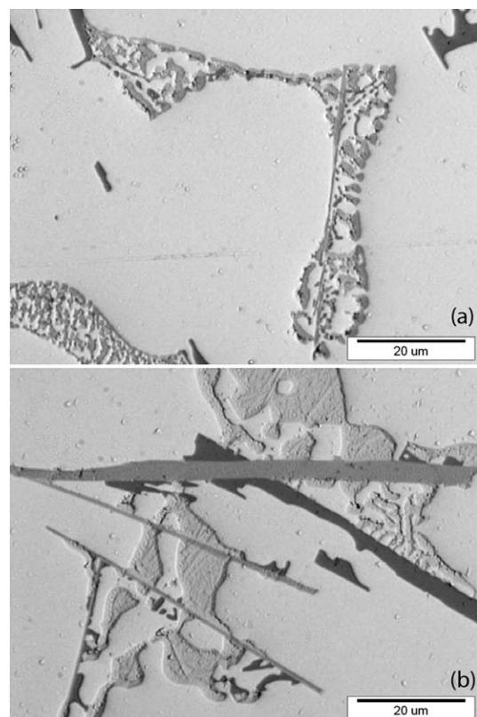
**Figure 7:** Microstructure of Al<sub>2</sub>Cu phase without Ce (a) and with  $w = 0.05\%$  Ce (b)
