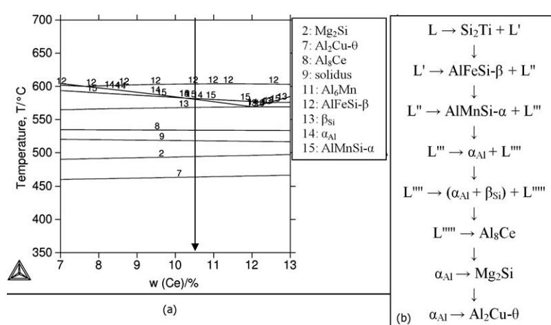
**Figure 1:** Equilibrium phase diagram (a) and schematic representation of equilibrium solidification of AlSi9Cu3 alloy (b) with  $w = 0.02\text{ \% Ce}$
