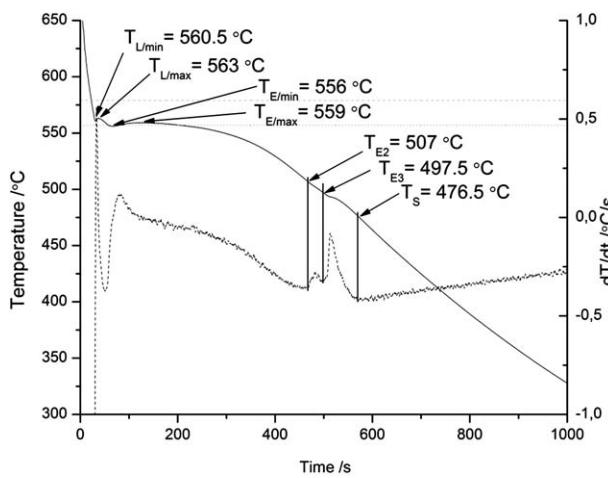
**Figure 2:** Cooling curve and differential cooling curve of AlSi9Cu3 alloy with  $w = 0.02\%$  Ce and with the theoretical calculated equilibrium liquidus and eutectic temperature (horizontal line)
