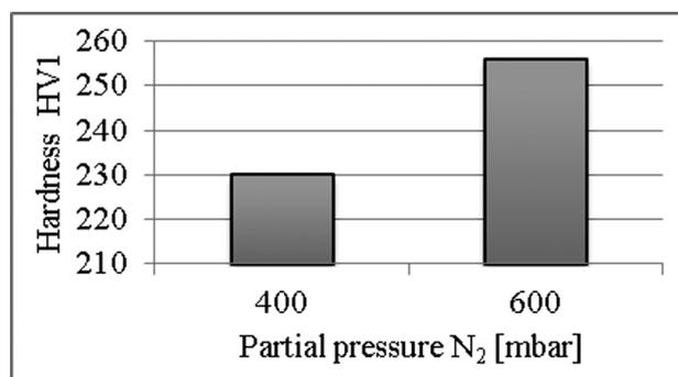
**Figure 4:** Influence of nitrogen partial pressure on the hardness of the sintered parts
