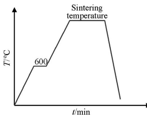
**Figure 1:** Thermal cycle of sintering and debinding
