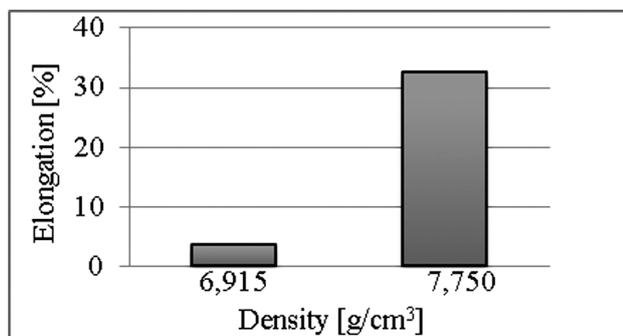
**Figure 3:** Influence of density on the elongation of the sintered parts
