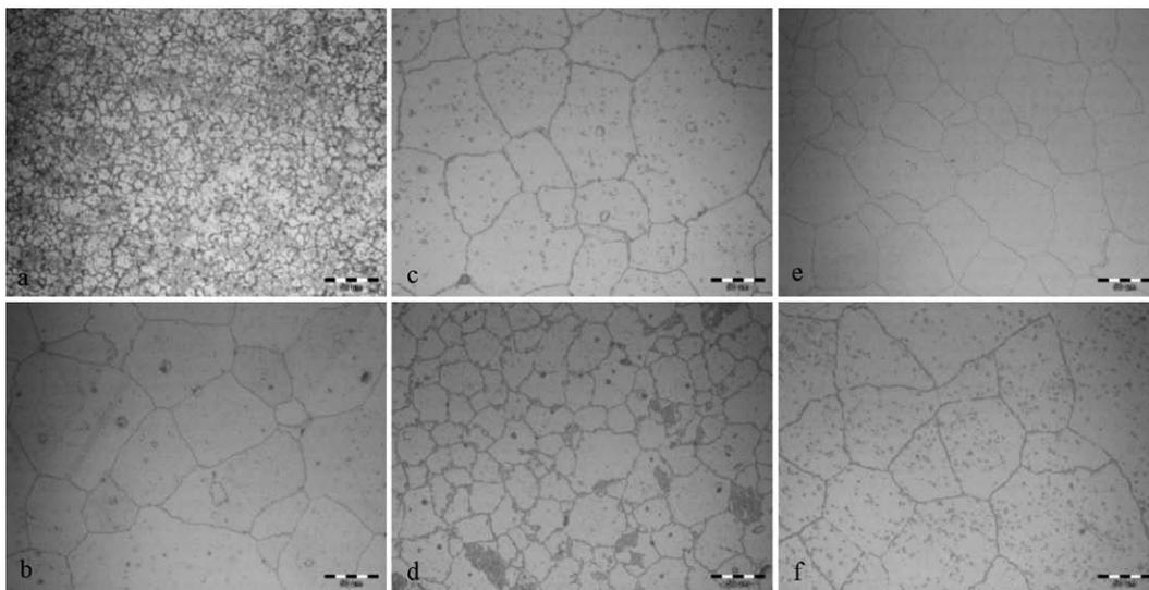
**Figure 5:** Microstructure of sintered parts for different conditions: a) argon, 1200 °C, 3 h, b) argon, 1310 °C, 3 h, c) argon, 1310 °C, 6 h, d) nitrogen, 1310 °C, 3 h, e) hydrogen, 1310 °C, 3 h, f) hydrogen, 1310 °C, 6 h, glyceregija
