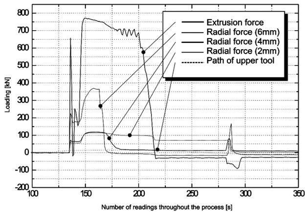
Figure 8: Force distribution at a die angle of 120°
