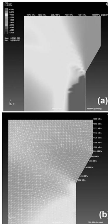
Figure 10: Contact stress at a die angle of 60°: a) on the punch and b) on the receiver wall in the radial direction
