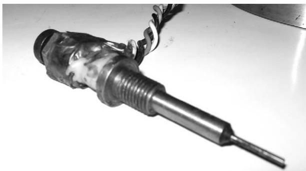
**Figure 2:** Measuring pin load-cell for radial forces
