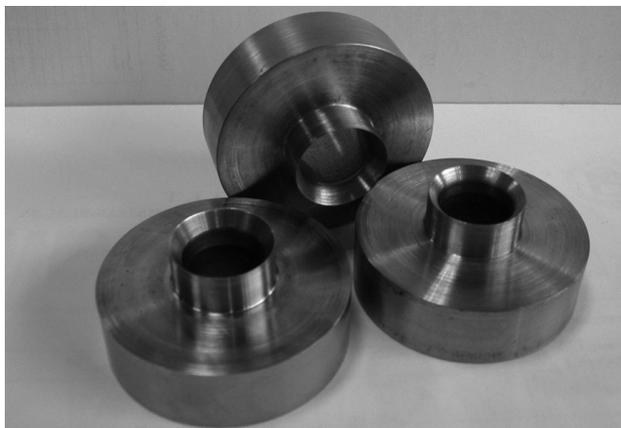
Figure 5: Extrusion matrices with various cone angles
