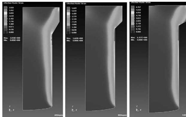
Figure 9: Field of effective plastic strain at three die angles: 60°, 90° and 120°
