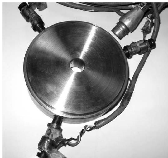
**Figure 4:** Experimental tool, receiver with three measuring pin load-cells
