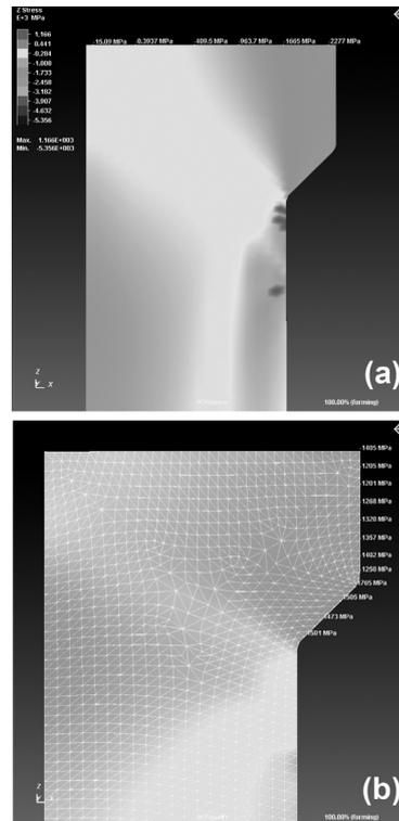
Figure 11: Contact stress at a die angle of 90°: a) on the punch and b) on the receiver wall in the radial direction
