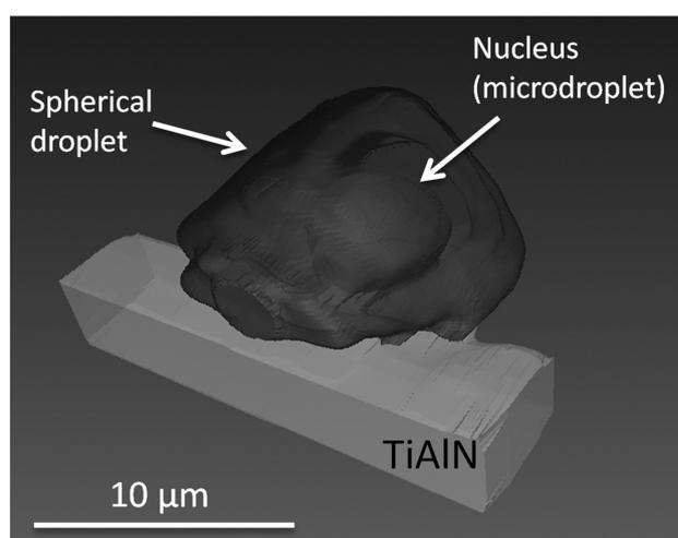
**Figure 4:** 3D-transparent image of a spherical droplet
