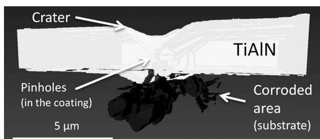
**Figure 3:** 3D reconstruction of a corrosion volume under a TiAlN coating on a site where a crater with pin holes was present
