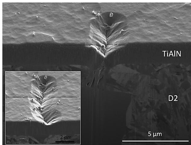
**Figure 1:** SEM image and FIB cross-sectional micrograph of the same growth defect (crater) on a sample TiAlN/D2 tool steel
