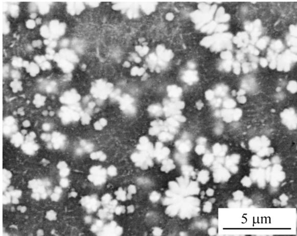
**Figure 1:** Microstructure of the as-cast ribbon, SEM-image. The coarser quasicrystals exhibit a characteristic dendritic morphology.
