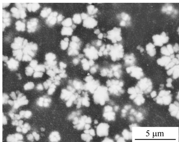
**Figure 4:** SEM micrograph of a sample after 24-h annealing at 400 °C: compared to the as-cast sample, no distinct changes can be observed.
