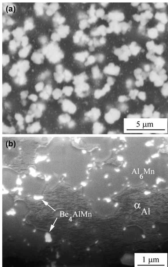
**Figure 5:** Ribbon annealed for 24 h at 550 °C: a) SEM back-scattered-electron image:  $\text{Be}_4\text{AlMn}$  and  $\text{Al}_6\text{Mn}$  can practically not be distinguished; b) FIB secondary-electron image of an in-situ prepared cross-section: all phases identified by XRD can be recognised
