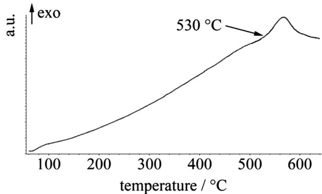
**Figure 3:** DSC curve of as-cast sample upon heating; heating rate 10 K min<sup>-1</sup>
