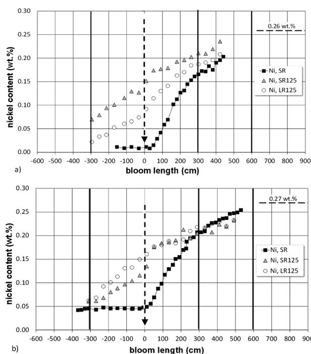
**Figure 2:** Graphic illustrations of the variations in the content of nickel on the surface and cross sections of CS No.5 blooms at a distance of 125 mm from the surface of round blanks in the casts using: a) a straight-through SEN and b) a five-port SEN
