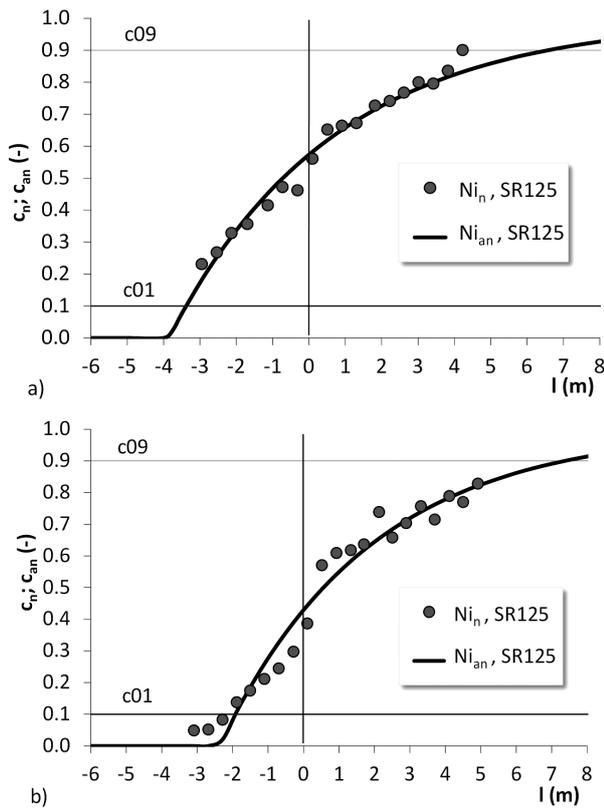
**Figure 5:** Approximation of the Ni-concentration variations on the cross sections of the CS No.5 blooms at a distance of 125 mm from the SR surface for: a) a straight-through and b) a five-port SEN
