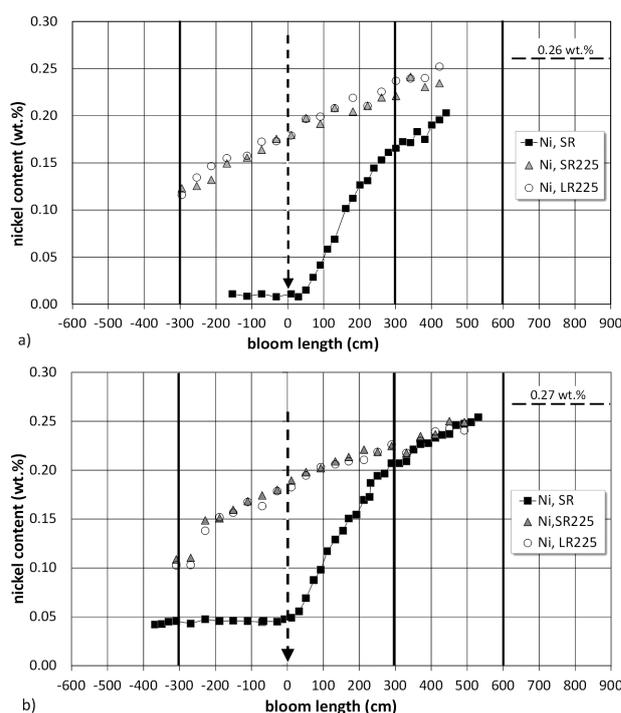
**Figure 3:** Graphic illustrations of the variations in the content of nickel on the surface and cross sections of CS No.5 blooms at a distance of 225 mm from the surface of the round blooms in the heats using: a) a straight-through SEN and b) a five-port SEN
