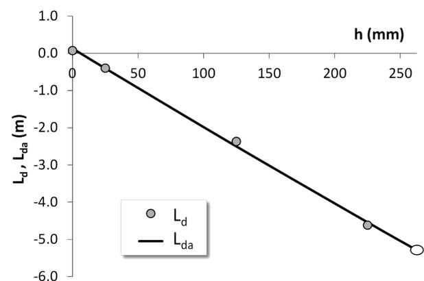
**Figure 7:** Approximative dependence of  $L_d$  on  $h$  for CS No.5 (with M-EMS), 5-port SEN, small radius
