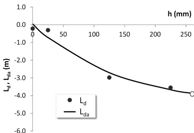
**Figure 6:** Approximative dependence of  $L_d$  on  $h$  for CS No.4, small radius, 5-port SEN
