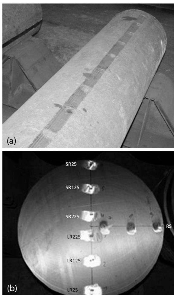
**Figure 1:** Separated blooms with a 525-mm diameter after spectrographic analyses: a) on the surfaces and b) on cross sections
