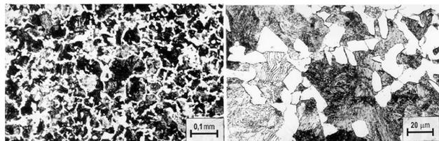
**Figure 3:** Microstructure of steel C45
