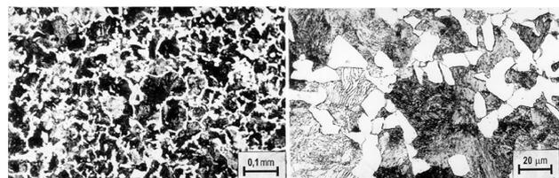
**Figure 3:** Microstructure of steel C45
