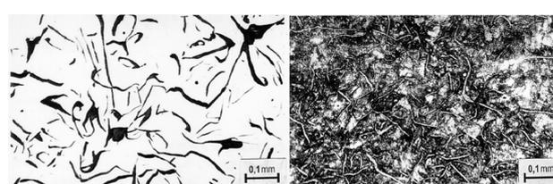
**Figure 6:** Microstructure of gray iron GJL200
