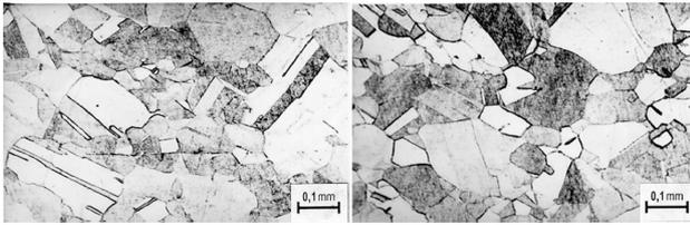
Figure 8: Microstructure of copper EK2-Cu.00
