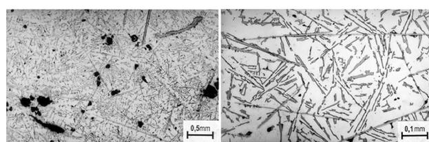
**Figure 7:** Microstructure of silumine AlSi<sub>12</sub>Cu.00
