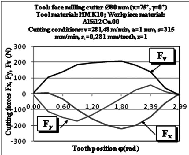
Figure 15:  $F_x$ ,  $F_y$  and  $F_v$  vs. tooth position – AlSi12Cu.00
