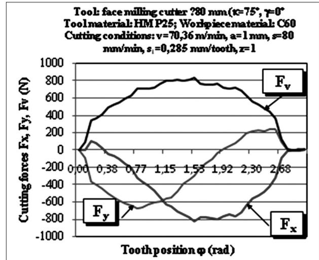
Figure 12:  $F_x$ ,  $F_y$  and  $F_v$  vs. tooth position – C60
