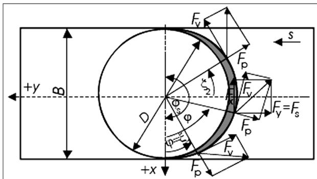
**Figure 1:** Scheme of cutting forces (Figure 1 in<sup>1</sup>)
