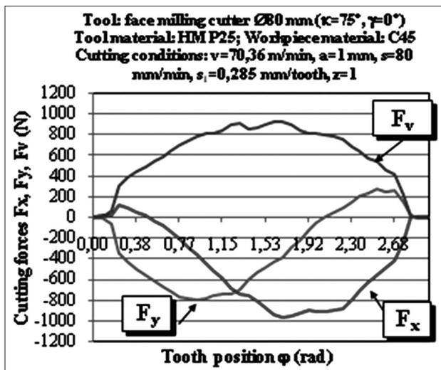
Figure 11:  $F_x$ ,  $F_y$  and  $F_v$  vs. tooth position – C45
