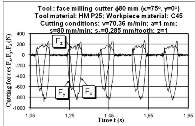
**Figure 2:** Cutting forces for five revolutions of the cutter
