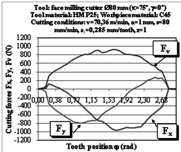
Figure 11:  $F_x$ ,  $F_y$  and  $F_v$  vs. tooth position – C45
