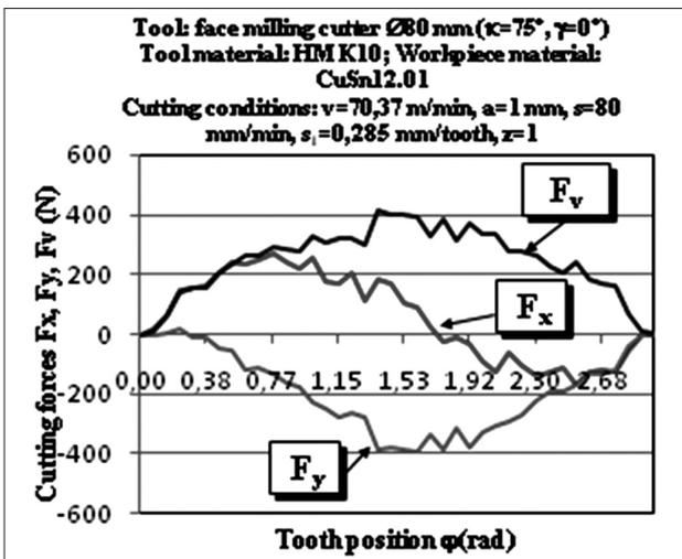
Figure 17:  $F_x$ ,  $F_y$  and  $F_v$  vs. tooth position – CuSn12.01
