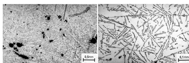
**Figure 7:** Microstructure of silumine AlSi<sub>12</sub>Cu.00
