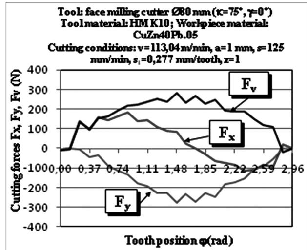
Figure 18:  $F_x$ ,  $F_y$  and  $F_v$  vs. tooth position – CuZn40Pb.05
