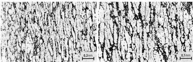
Figure 10: Microstructure of brass CuZn40Pb.05
