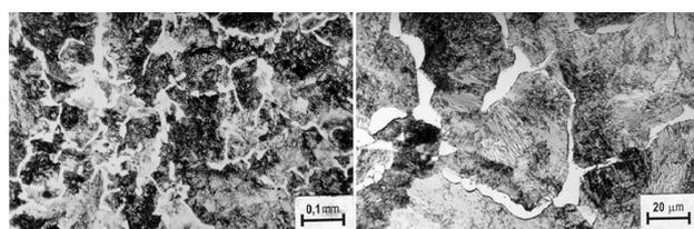
**Figure 4:** Microstructure of steel C60
