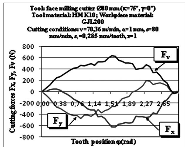
Figure 14:  $F_x$ ,  $F_y$  and  $F_v$  vs. tooth position – GJL200
