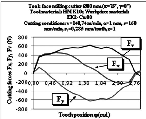
Figure 16:  $F_x$ ,  $F_y$  and  $F_v$  vs. tooth position – EK2-Cu.00
