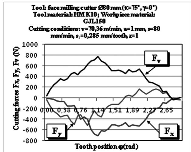
Figure 13:  $F_x$ ,  $F_y$  and  $F_v$  vs. tooth position – GJL150
