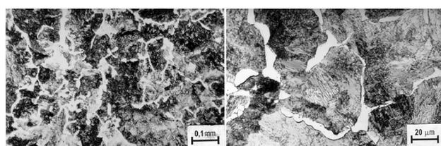
**Figure 5:** Microstructure of gray iron GJL150
