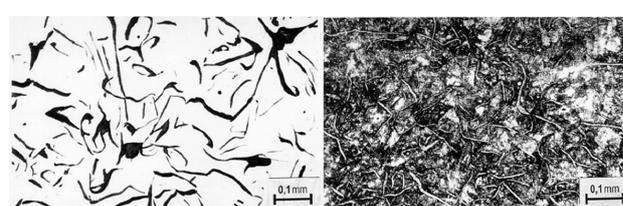
**Figure 6:** Microstructure of gray iron GJL200
