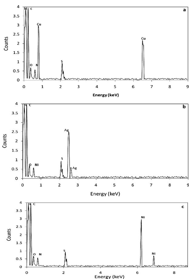
**Figure 2:** Typical EDS analysis of a nanoparticle: a) poly(DDS)-Cu, b) poly(DDS)-Ag, c) poly(DDS)-Ni composite materials
