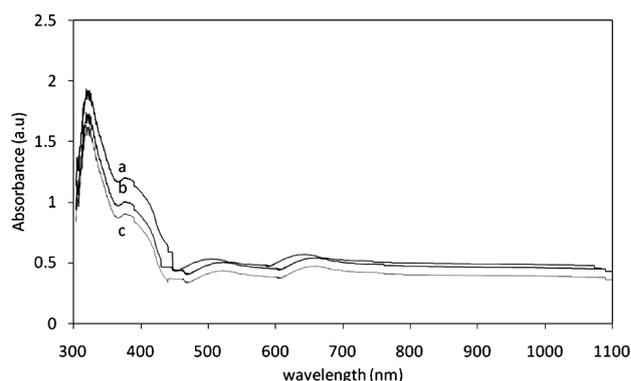
**Figure 3:** UV-vis spectrum of the metal-polymer composite material: a) polymer-Cu, b) polymer-Ni, c) polymer-Ag
