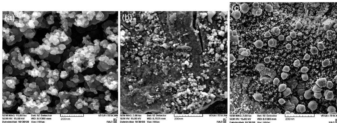
**Figure 1:** SEM image of the: a) poly(DDS)-Cu, b) poly(DDS)-Ni, c) poly(DDS)-Ag composite materials
