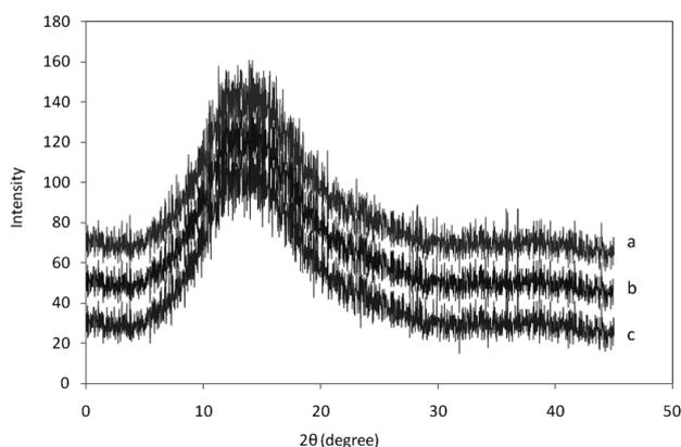
**Figure 5:** X-ray diffraction patterns of: a) polymer-Cu, b) polymer-Ni and c) polymer-Ag
