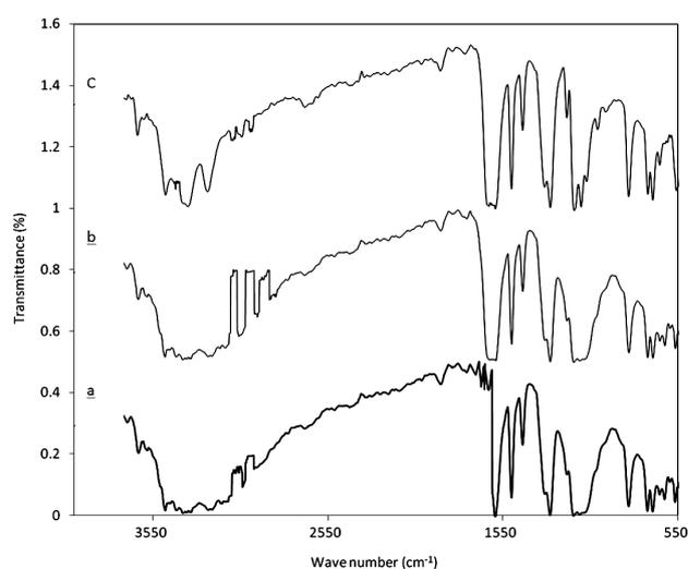
**Figure 4:** IR spectrum of the composite material: a) polymer-Ag, b) polymer-Cu, c) polymer-Ni
