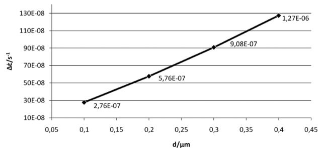
**Figure 2:** Dependence of creep rate increase versus particles size during an increase of temperature from 540 °C to 630 °C
