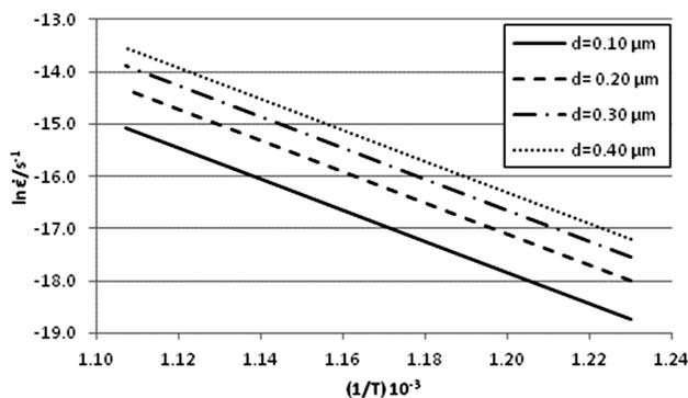
**Figure 3:** Arrhenius dependence in temperature range 540 °C to 630 °C for different particle sizes
