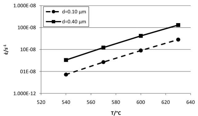
**Figure 1:** Dependence of accelerated creep rate versus temperature for particle sizes 0.10 μm and 0.40 μm
