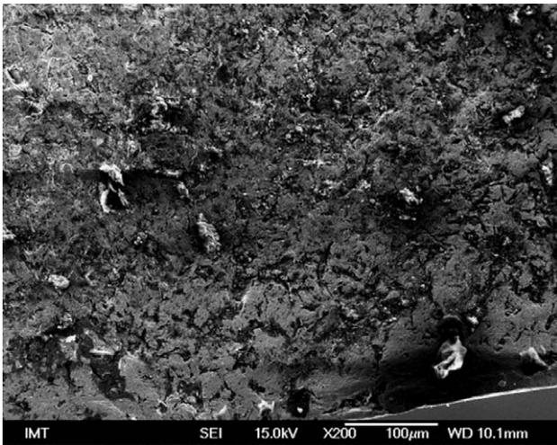
**Figure 10:** SEM image of plastically deformed surface area 1.1
