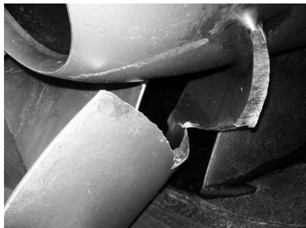
Figure 2: Damaged impeller blade
