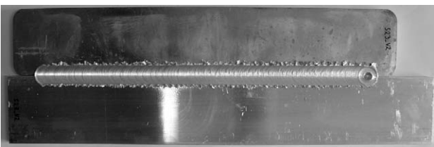
Figure 5: Plates joint with FSW (upper plate of AA413.0 alloy, lower plate of AA1050 alloy) Slika 5: Plošči, spojeni s FSW-spojem (zgoraj zlitina AA413.0, spodaj zlitina AA1050)
