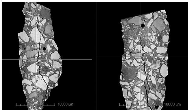
**Figure 3:** Vertical cross-sections of a piece of concrete approximately 3.0 cm in size. The cementitious matrix, at least two types of aggregate grains, air voids and cracks are presented in the image with different greyscale values.
