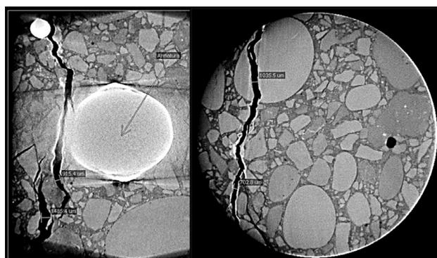
**Figure 1:** 2D slice in the XY direction of the steel bar embedded in the concrete (left image). A layer of the secondary corrosion products is visible on the surface of the embedded bar (the bright layer) as well as on the surface of the newly formed crack (left and right image). The cracks in the concrete cover were formed due to the increased volume of the secondary corrosion products.
