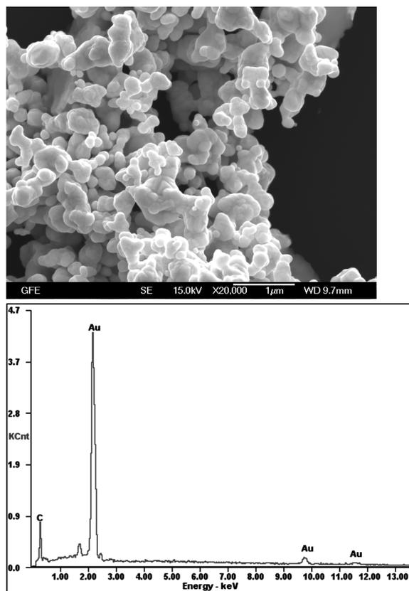
**Figure 2:** SEM image and EDS analysis of the Au nanoparticles obtained in an ultrasonic generator
