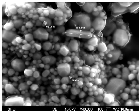
**Figure 5:** SEM image of Au nanoparticles (synthesis parameters: 280 °C, 2.5 MHz)
