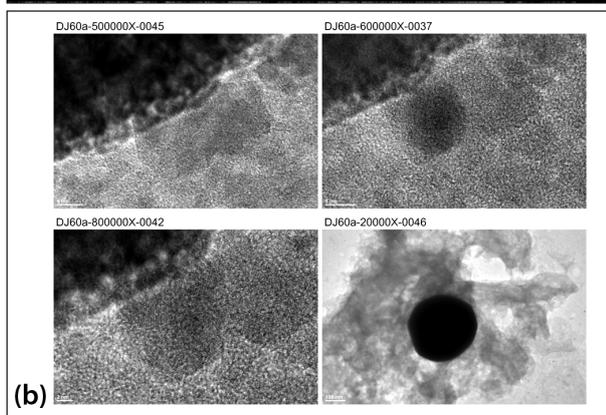
**Figure 3:** a) SEM image of Au nanoparticles (synthesis parameters: 260 °C,  $f = 0.8$  MHz), b) TEM image of Au nanoparticles (synthesis parameters: 260 °C,  $f = 0.8$  MHz)
