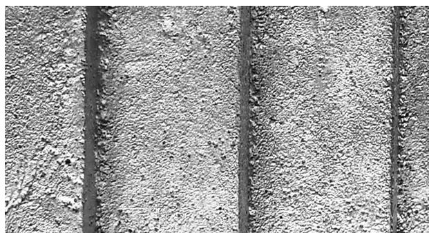
**Figure 6:** Appearance of the mullite-based lining on a test sample without visible flaws
