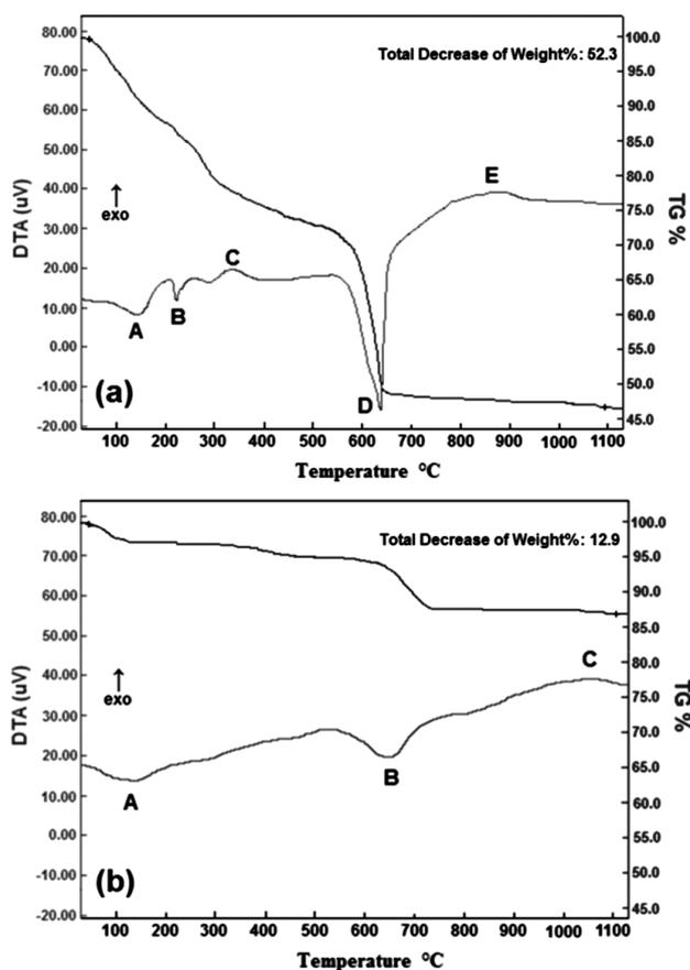
**Figure 2:** DTA and TG curves of SrZn<sub>2</sub>Si<sub>2</sub>O<sub>7</sub> gels from 25 °C up to 1150 °C for: a) SG and b) SS samples
