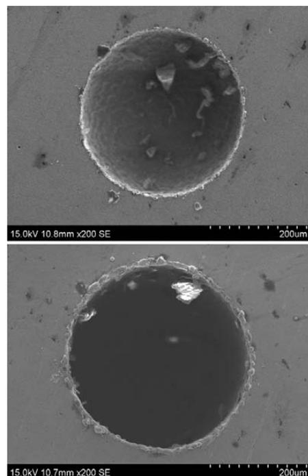
**Figure 1:** SEM image of a micro-hole on the workpiece
