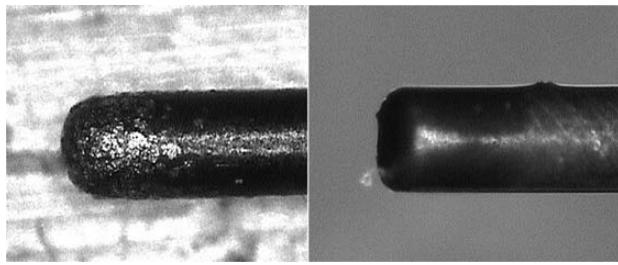
**Figure 2:** VMS image of the electrode after machining
