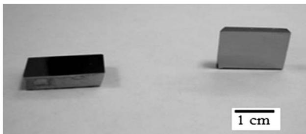
**Figure 1:** Transverse and longitudinal section of hardened material
