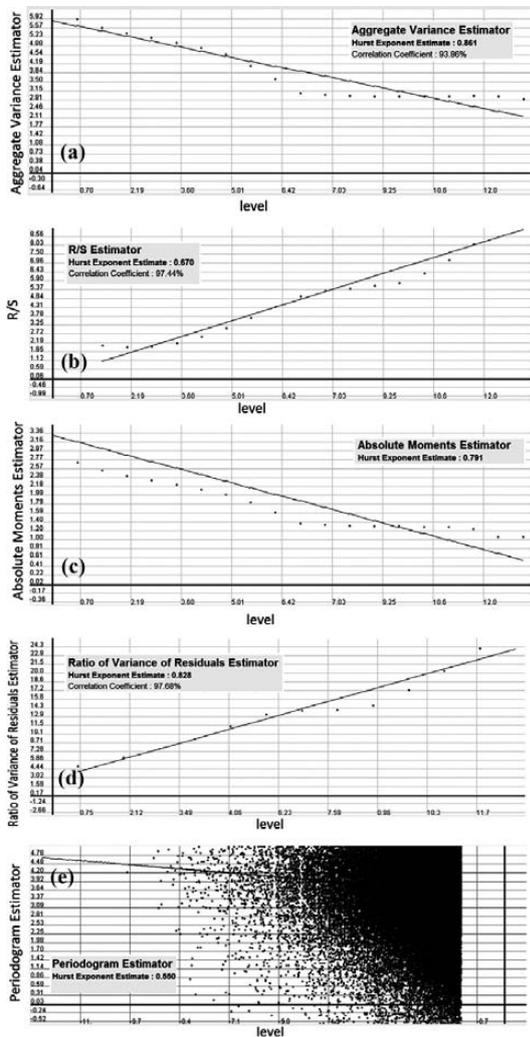
**Figure 11:** a) Variance method for hardened material 1.7225, b) R/S method for hardened material 1.7225, c) Absolute moments estimator for hardened material 1.7225, d) Variance of residuals method for hardened material 1.7225, e) Periodogram method for hardened material 1.7225
