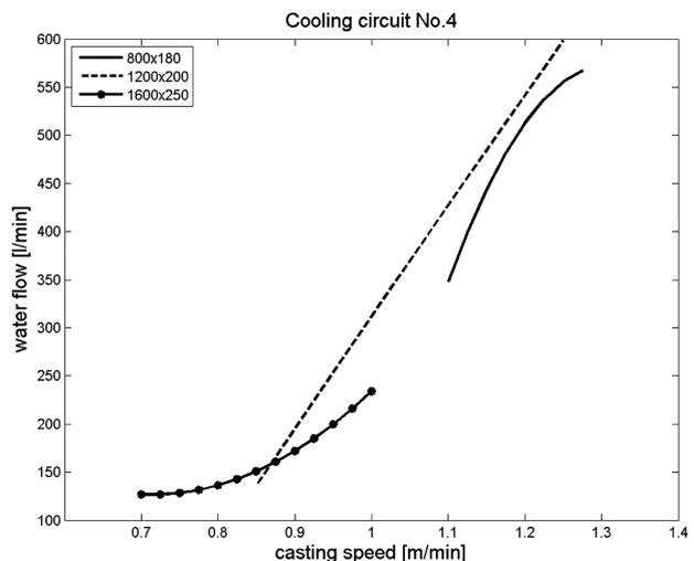
Figure 5: Optimal cooling curves for cooling circuit No. 4
