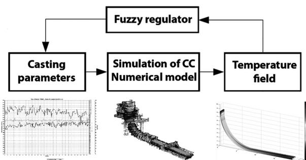
**Figure 1:** Block scheme of the regulation approach
