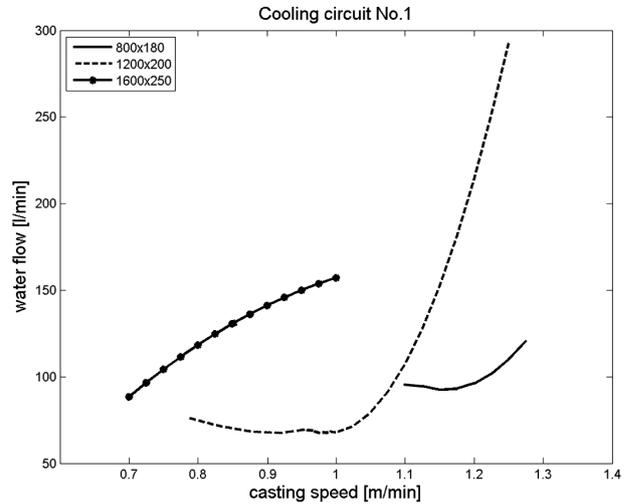
Figure 4: Optimal cooling curves for cooling circuit No. 1
