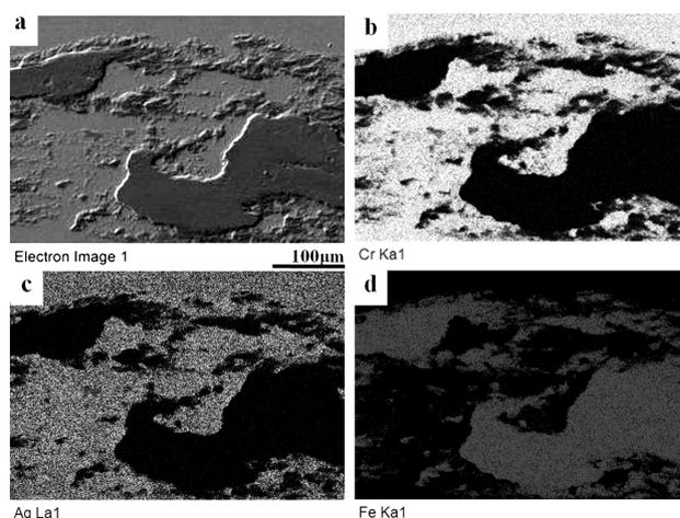
**Figure 7:** Material transferred from counterpart 100Cr6 to the surface of coating CrAg7N after pin-on-disc, at the temperature 20 °C: a) overview, b) EDX of chromium, c) EDX of silver, d) EDX of iron
