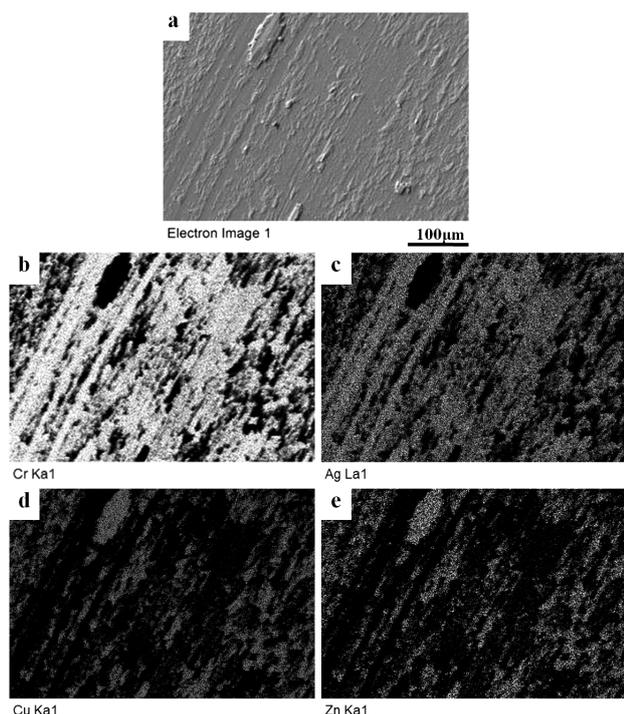
**Figure 6:** Material transferred from counterpart CuZn to the surface of coating CrAg7N after pin-on-disc, at the temperature of 20 °C: a) overview, b) EDX of chromium, c) EDX of silver, d) EDX of copper, e) EDX of zinc
