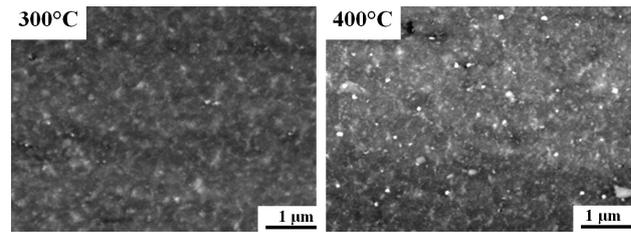
**Figure 4:** Nanoparticles of silver on the surface of track after pin-on-disc testing
