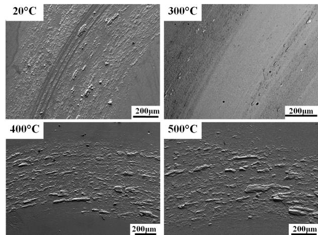
**Figure 5:** Wear tracks after pin-on-disc testing against CuZn at ambient and elevated temperature
